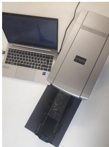
Figure 3. High-resolution Reflecta scanner connected to Silverfast and Fibershape software.
