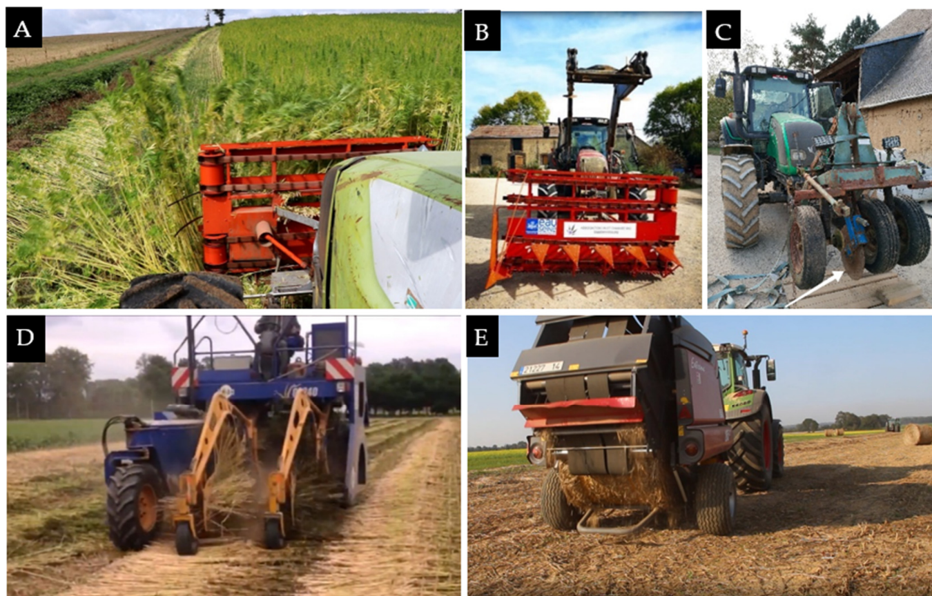
Figure 1. Machines for hemp cultivation. (A,B): Single-bar mower. (C): Cutting disc machine. (D): Flax returning machine. (E): Flax baling machine.
