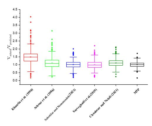
**Figure 8.** A box plot illustrating the distribution of actual-to-predicted strength ratios for the shear strength of SFRC beams [35,54,61,63,64].
