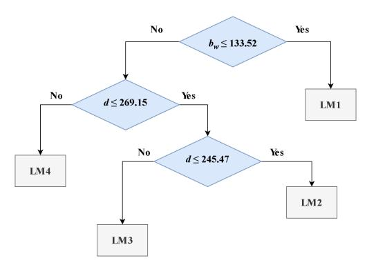
Figure 2. M5P algorithm tree for estimating the shear strength of SFRC beams.
