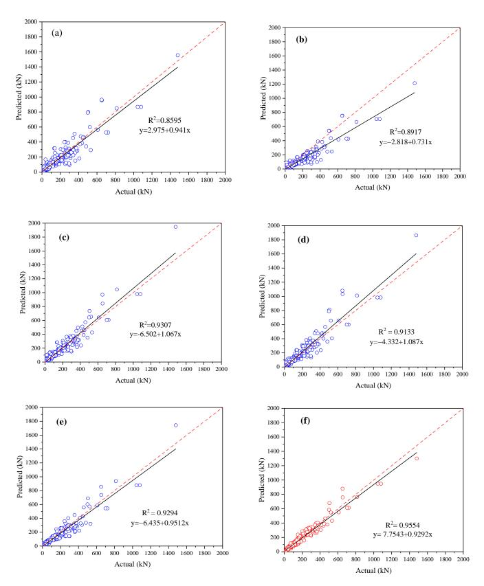
**Figure 6.** Comparison of shear strength between experimental outcomes and various computational techniques: (a) Ashour et al. [61], (b) Khuntia et al. [54], (c) Sabetifar and Nematzadeh [35] (d) Sarveghadi et al. [63], (e) Chaabene and Nehdi [64], (f) proposed M5P model.
