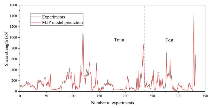
**Figure 4.** Comparison of the predictions generated by the M5P-tree-based model with the experimental measurements of the shear strength for both training and testing datasets.
