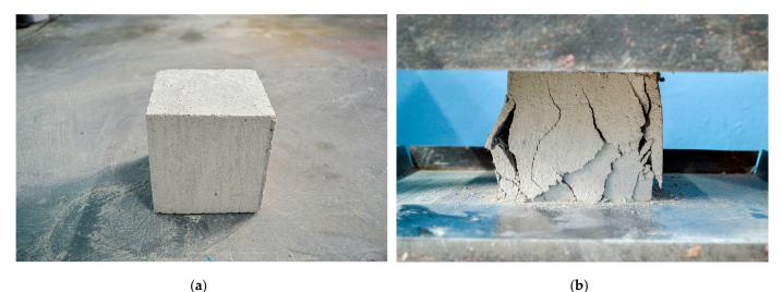
Figure 5. Sample of aerated concrete modified with GGBS and reinforced with SF: (a) before the compression test; and (b) after the compression test.
