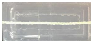
Figure S1 † The single-line-knotted fiber for surface ZP measurement.
