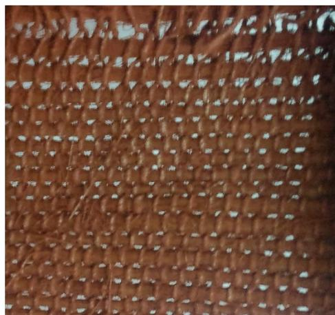
**Figure 8.** Iron oxide-coated sisal fiber-based filter media.
