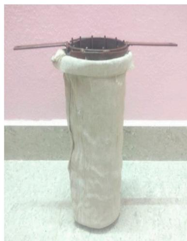
Figure 3. Zinc oxide-coated sisal fiber-based filter media.
