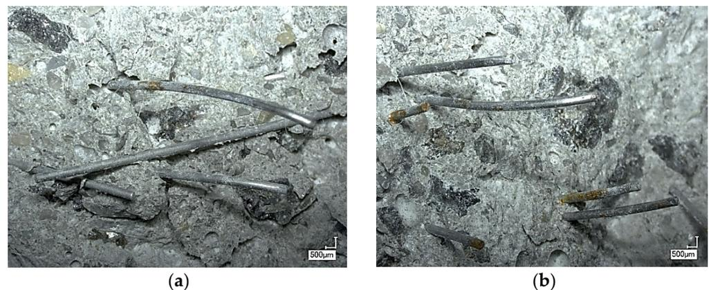
**Figure 7.** (a,b) Microscopic view of the rupture surfaces for SF and short PP fiber in the concrete matrix.
