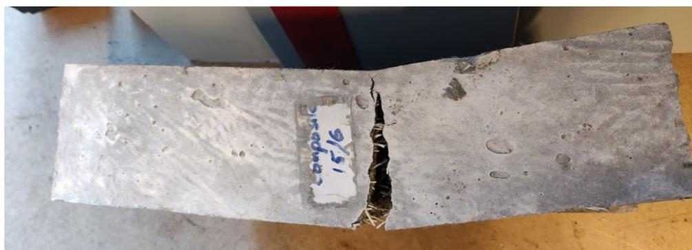
**Figure 4.** Tested FRC sample.
