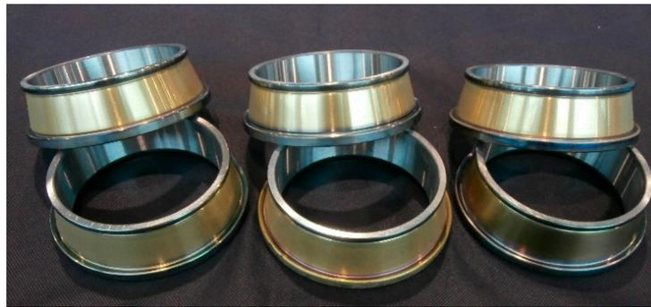
Figure 13. Bearing samples D4 coating + B polish post-processing.
