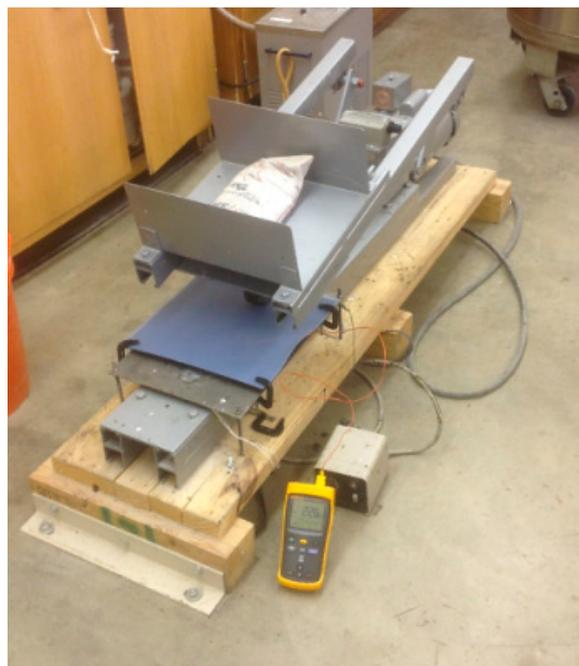
**Figure 2.** Diagram of the modified loaded wheel test (MLWT).
