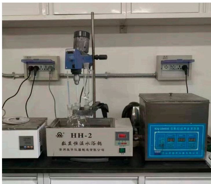
Figure 1. The experiment set-up of the SiO 2 · n H 2 O nanoparticles synthesis.
