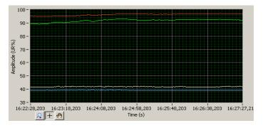
**Figure 11.** The graph representing the variation of the relative humidity of the wet stream (entry in red and exit in green) and of the dry stream (entry in light blue and exit in gray).
