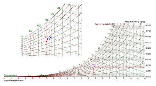
**Figure 17.** Psychrometric diagram representing the variation of the thermo-hygrometric state of cold and dry flow in cross-linked SPEEK (DXL = 0.1).
