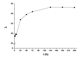
**Figure 7.** Equilibrium water uptake coefficients ( $\lambda$ ) vs. time for a sample treated at 120–24 and 180–10 with final DS = 0.73, ion exchange capacity (IEC) = 2.1 and crosslinking degree (DXL) = 0.22.
