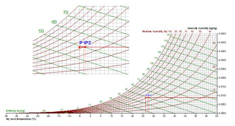
**Figure 13.** Psychometric diagram representing the variation of the thermohygrometric state of cold and dry flow in a plastic material.
