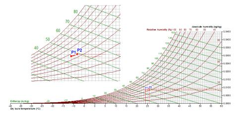
**Figure 15.** Psychrometric diagram representing the variation of the thermohygrometric state of the cold and dry flow in Nafion<sup>™</sup> NRE-212.
