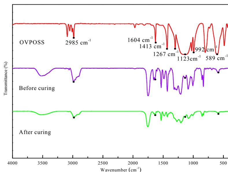
**Figure 2.** The infrared spectra of octavinyl polyhedral oligomeric silsesquioxane (OVPOSS) hybrid coating before and after curing.
