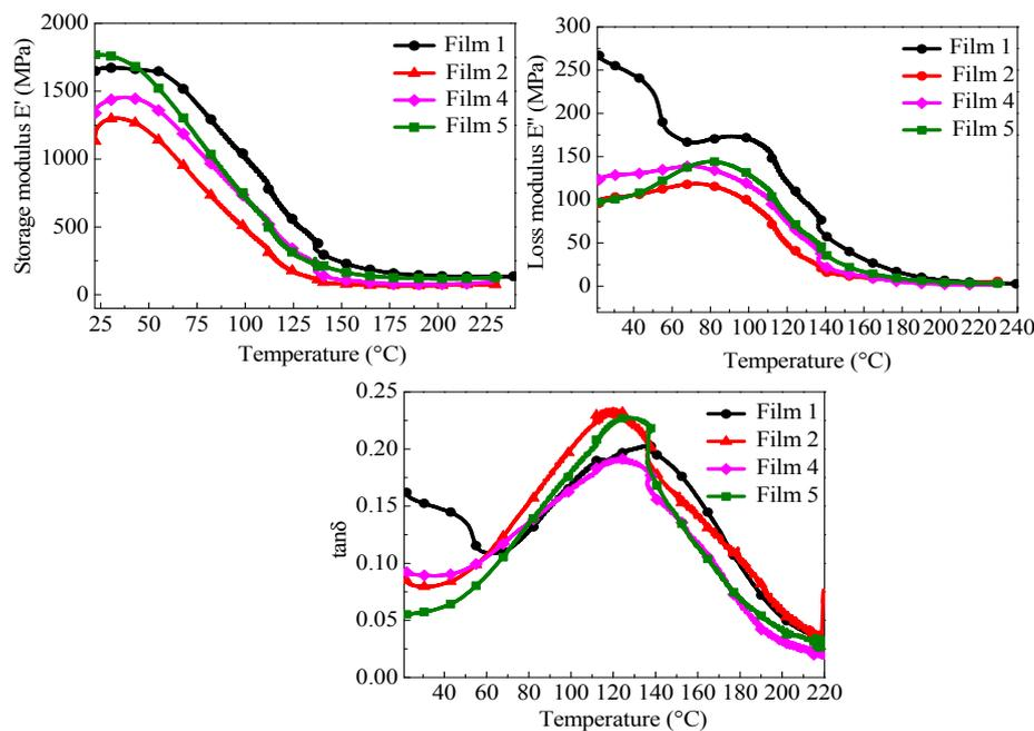
**Figure 4.** The effect of different inorganic materials on the storage modulus ( $E'$ ), loss modulus ( $E''$ ), and  $\tan \delta$  curve of the coatings.
