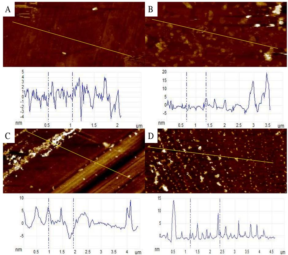
**Figure 7.** AFM 2D images and their corresponding height profiles of organic and composite coatings: (A) Film 1; (B) Film 2; (C) Film 4; (D) Film 5.
