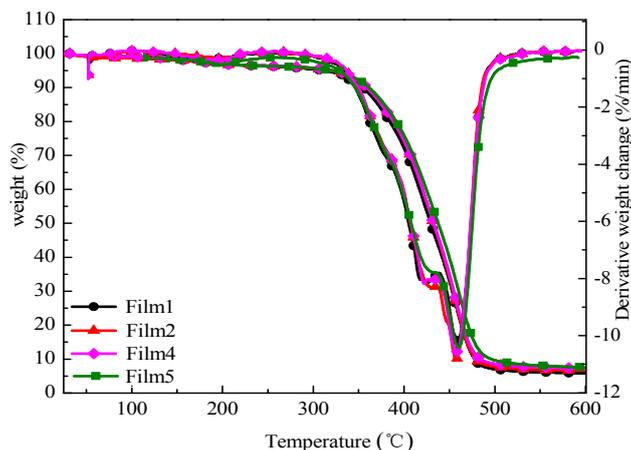
**Figure 3.** Thermal gravity (TG) and differential TG (DTG) curves of pure organic and composite coatings.
