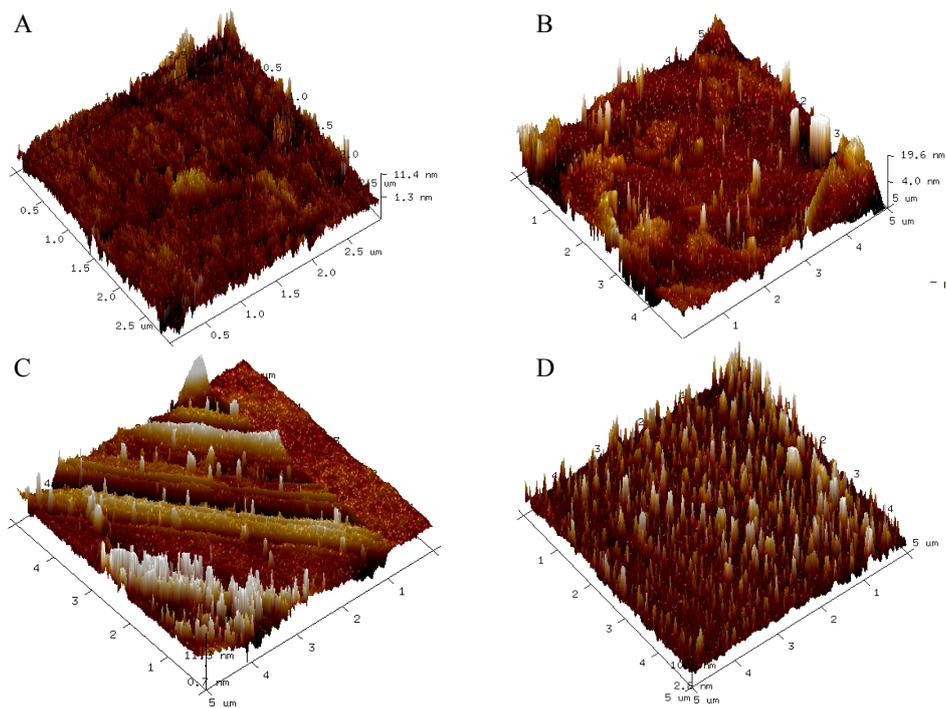
**Figure 6.** Atomic force microscope (AFM) 3D images of organic and composite coatings: (A) Film 1; (B) Film 2; (C) Film 4; (D) Film 5.
