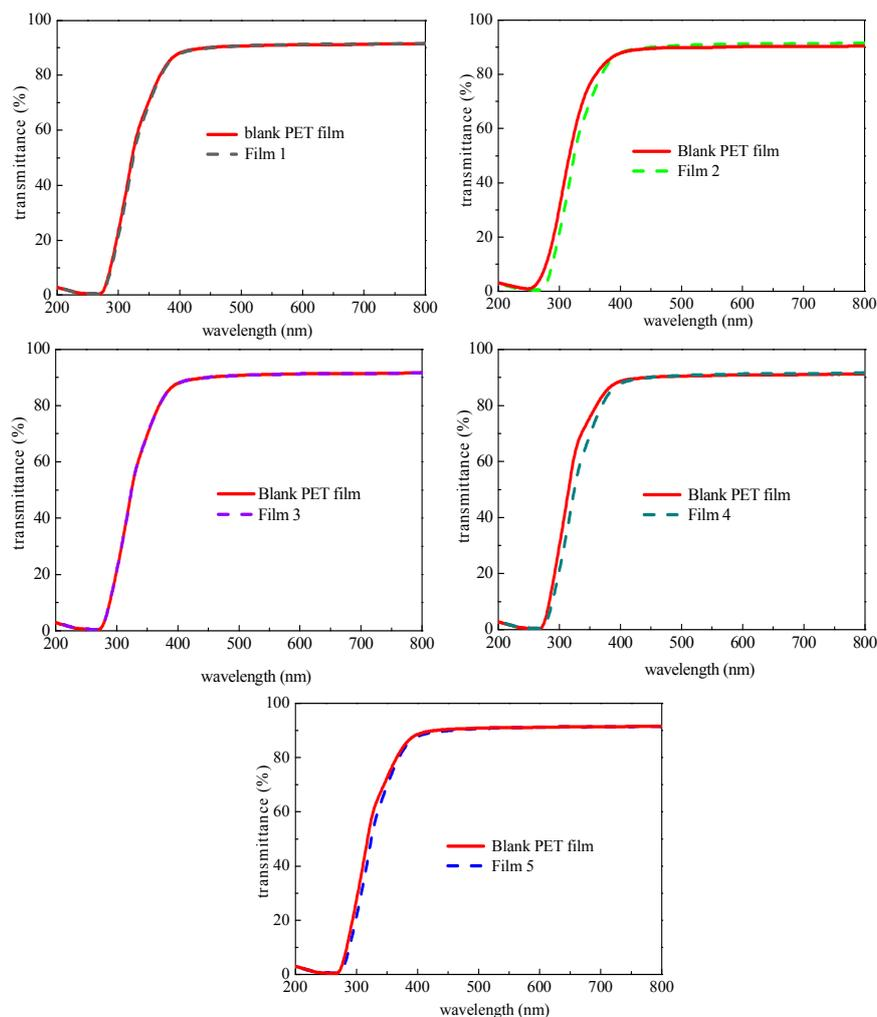
**Figure 1.** Effect of different nanoparticles on the transmittance of UV-cured films.
