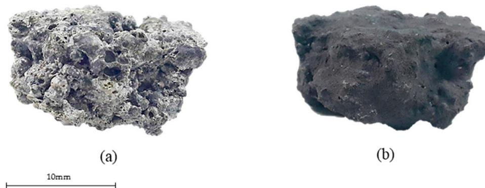
Figure 8. POC particle: (a) Pre-coating; (b) After coating.
