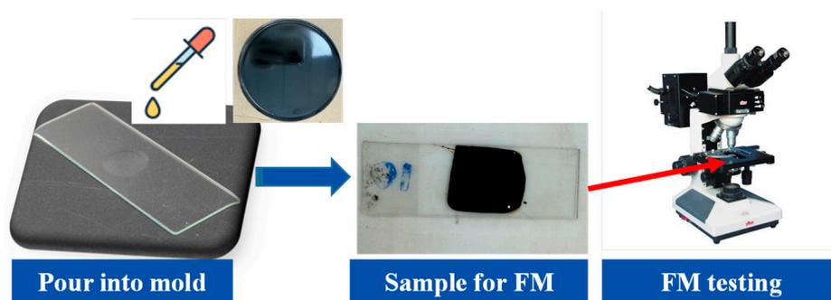
**Figure 3.** Fluorescence microscopy of asphalt.
