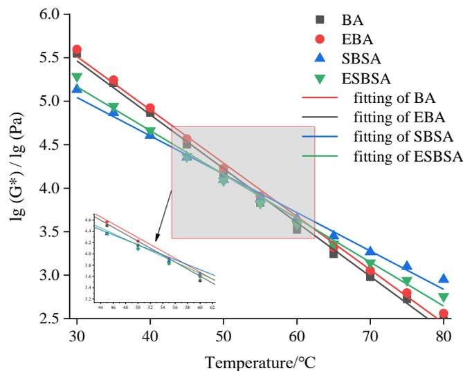
**Figure 5.** Fitting curve of asphalt composite modulus-temperature before and after emulsification.
