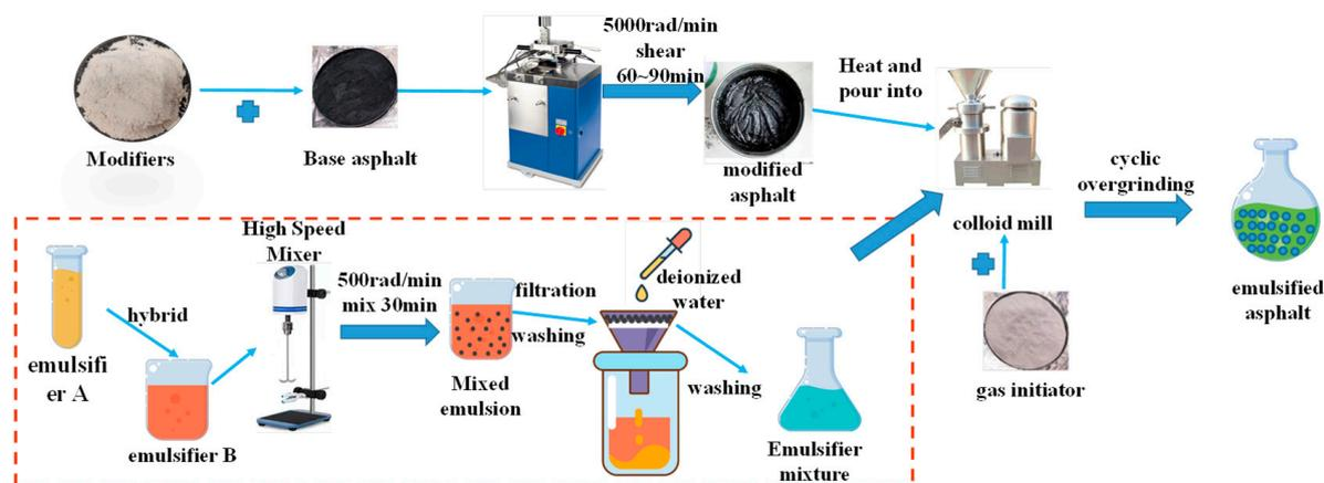
**Figure 1.** Flow chart of emulsified asphalt preparation.
