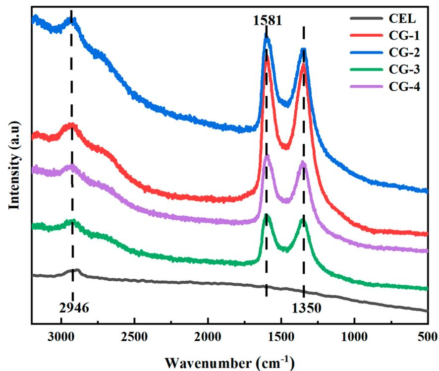
Figure 3. CEL-GO composite gas gel Raman spectroscopy analysis.
