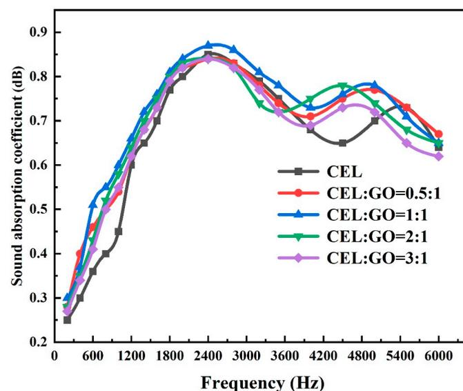
Figure 7. Sound absorption performance analysis of CEL-GO composite aerogel.
