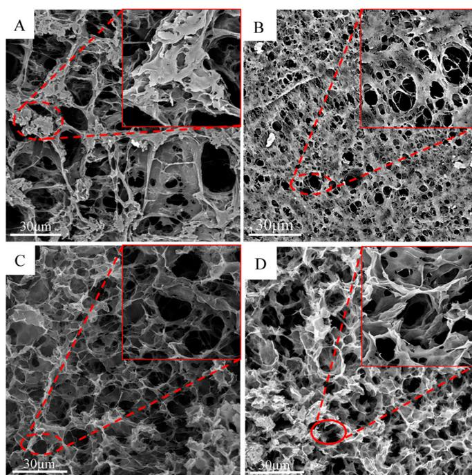
**Figure 4.** SEM analysis of CEL-GO composite aerogel. Pictures (A–D) correspond to aerogels in the ratios CEL:GO = 0.5:1; CEL:GO = 1:1; CEL:GO = 2:1; CEL:GO = 3:1.
