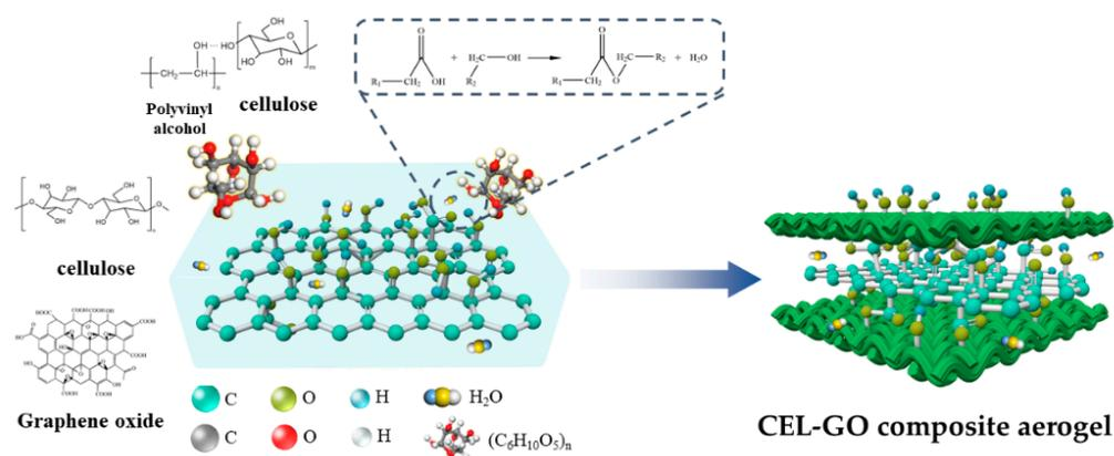
**Figure 8.** The molecular structure model of sound absorption mechanism of CEL-GO composite aerogel.
