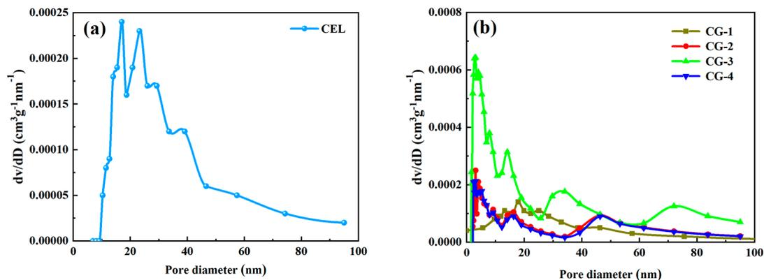
**Figure 6.** (a) CEL aerogel pore size distribution curve; (b) CEL-GO composite aerogel pore size distribution curve aerogel.
