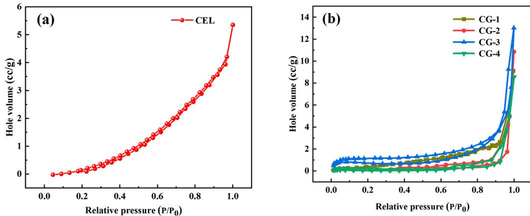
**Figure 5.** Aerogel nitrogen adsorption–desorption test: (a): CEL aerogel; (b): CEL-GO composite aerogel.
