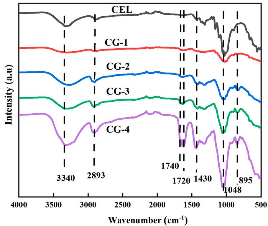
Figure 2. Infrared spectroscopy of CEL and CEL-GO composite aerogels.
