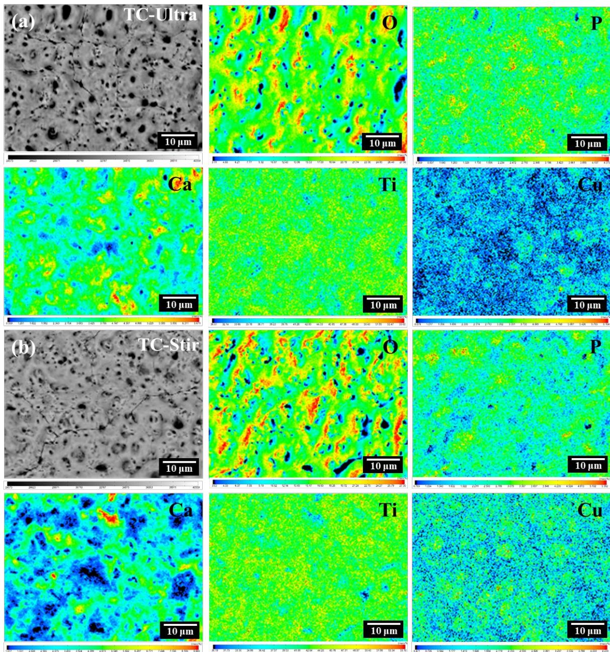
**Figure 3.** EPMA analysis of coating surfaces: (a) SEM micrograph of TC-ultra with the corresponding EDX maps in sequence of Ti, Cu, O, P, and Ca; (b) SEM micrograph of TC-stir with the corresponding EDX maps in sequence of Ti, Cu, O, P, and Ca.
