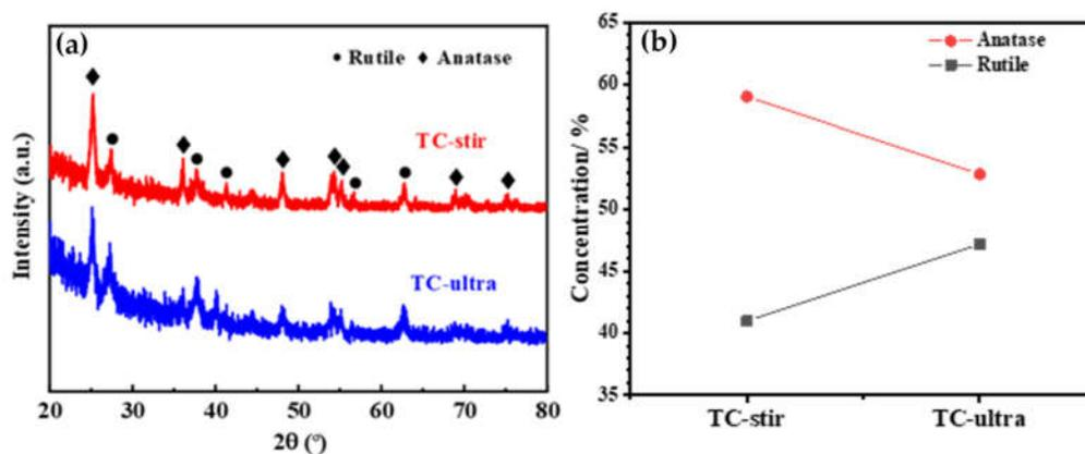
Figure 6. TFXRD patterns (a) and concentration (%) of rutile and anatase phases (b) of TC-stir and TC-ultra.
