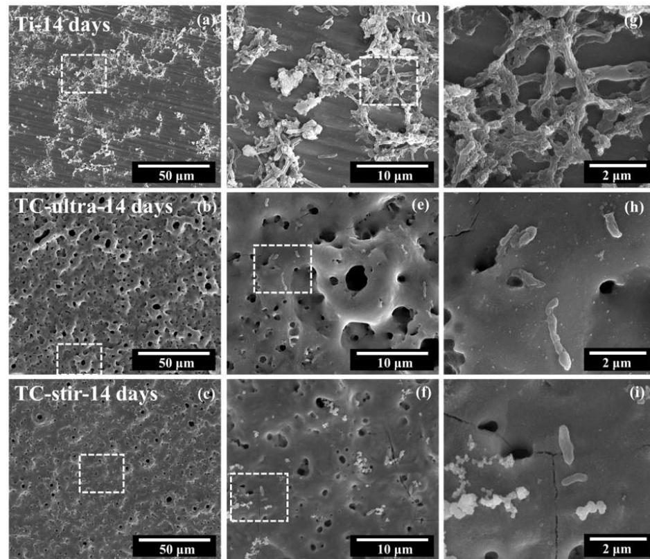
**Figure 10.** SEM micrographs of SRB on the surfaces of both Cu-modified TiO<sub>2</sub> coatings with metallic Ti as a comparison after immersion for 14 days: (a,d,g) Ti, (b,e,h) TC-ultra and (c,f,i) TC-stir.
