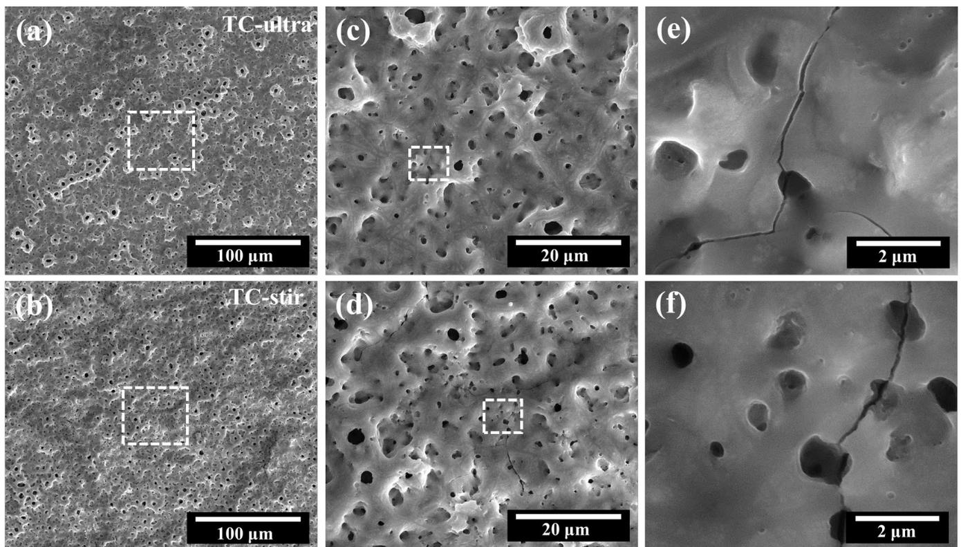
**Figure 2.** SEM micrographs of coating surfaces: (a,c,e) TC-ultra; (b,d,f) TC-stir.
