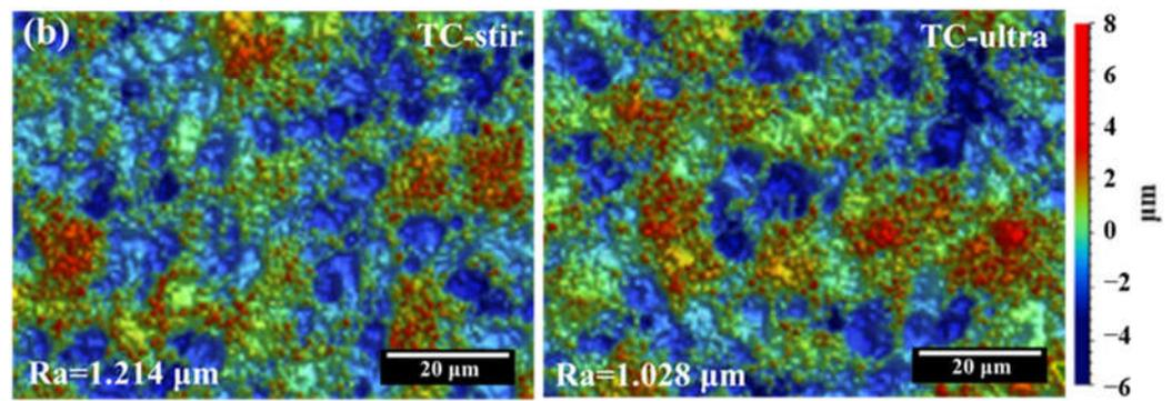
Figure 8. (a) Water contact angles and (b) surface topography for both Cu-modified TiO<sub>2</sub> coatings.
