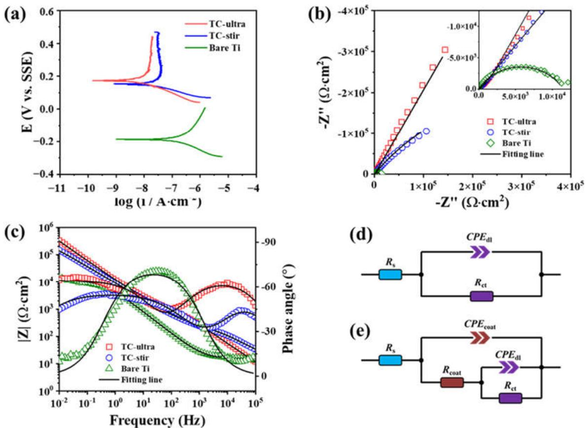
Figure 9. Electrochemical measurements for TC-stir and TC-ultra: (a) potentiodynamic polarization curves; (b) Nyquist plots of EIS; (c) Bode plots of EIS; and (d,e) equivalent circuit (EC) model for EIS.
