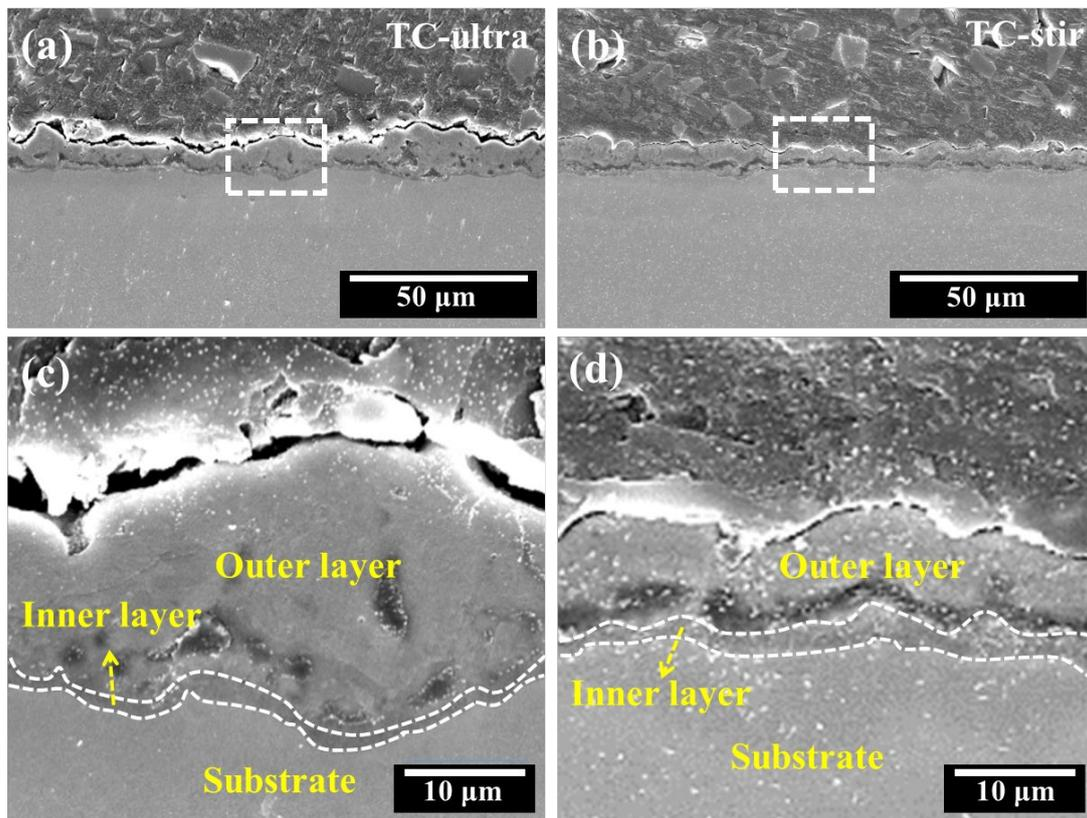
**Figure 4.** SEM micrographs of cross-sectional views in the coatings: (a,c) TC-ultra; (b,d) TC-stir.
