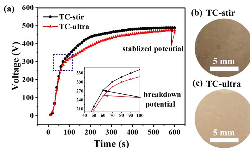
**Figure 1.** (a) Voltage–time curves during the micro-arc oxidation with and without the introduction of ultrasonic vibration; (b,c) surface appearances of both coatings.
