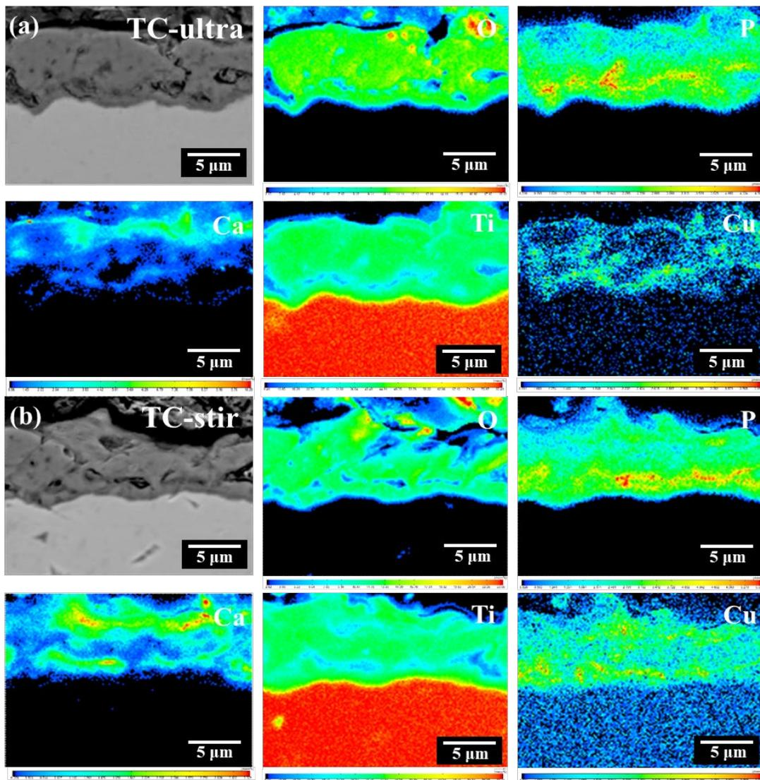
Figure 5. EPMA analysis of cross sections in both Cu-modified TiO<sub>2</sub> coatings: (a) TC-ultra, (b) TC-stir.
