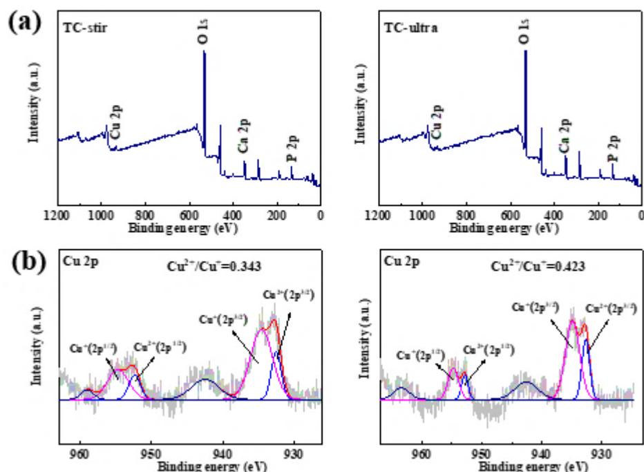
Figure 7. (a) XPS surveys; (b) high-resolution XPS spectra of Cu in both Cu-modified TiO<sub>2</sub> coatings.
