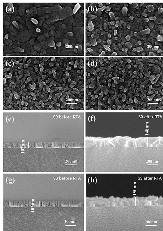
**Figure 8.** SEM photographs of VO<sub>2</sub> films with different Ti contents. (a–d) Samples with sputtering times from 0 to 6 min and Ti surface dopant contents from 0% to 0.43%, respectively; (e–h) the cross-sections of samples before and after rapid thermal annealing (RTA) [59]. (Reused with permission from ref. [59]. Copyright 2022, Elsevier).
