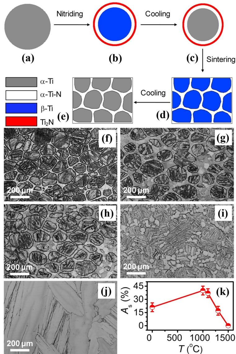
**Figure 4.** The formation process of the core-shell Ti-N alloys during the nitriding (a–c) and SPS sintering (c–e) processes. Microstructure variation of the SPS-sintered specimen: (f) before annealing; (g–j) those annealed under 1000, 1100, 1300, and 1500 °C; (k) variations of shell area fraction  $A_s$  versus annealing temperature  $T$ . [40] (Reused with permission from ref. [40]. Copyright (2017), Springer Nature).
