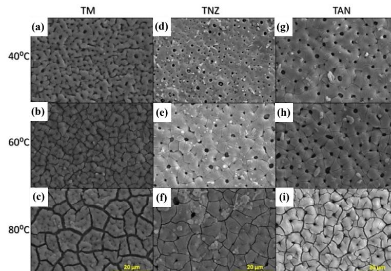
**Figure 7.** SEM images of Ti-15Mo (TM) (a–c), Ti-13Nb-13Zr (TNZ) (d–f), and Ti-6Al-7Nb (g–i) samples after anodization and immersion in 5 M NaOH at various temperatures for 8 h. [55] (Reused with permission from ref. [55]. Copyright 2017, MDPI).
