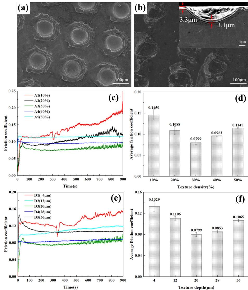
**Figure 3.** SEM image and EDS analysis of samples: (a) textured titanium alloy sample; (b) textured diamond-like carbon (DLC)-coated sample. Friction coefficient of samples with different texture densities; (c) friction coefficient curve; (d) average value of friction coefficient; different texture depths; (e) friction coefficient curve; and (f) average value of friction coefficient [35] (Reused with permission from ref. [35]. Copyright 2020, IOP Publishing).
