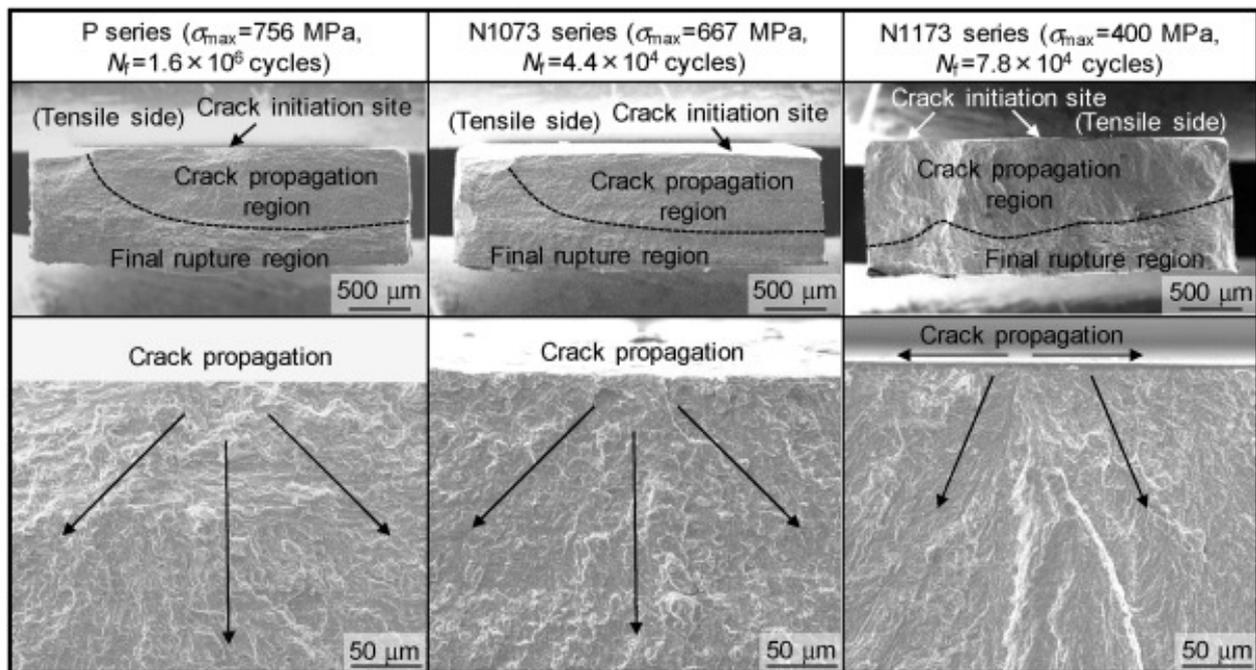
**Figure 5.** SEM micrographs of the fractured surfaces of failed specimens that were polished (P series) and induction-heated at 1073 K (N1073 series) and 1173 K (N1173 series) in nitrogen [42]. (Reused with permission from ref. [42]. Copyright 2020, Elsevier).
