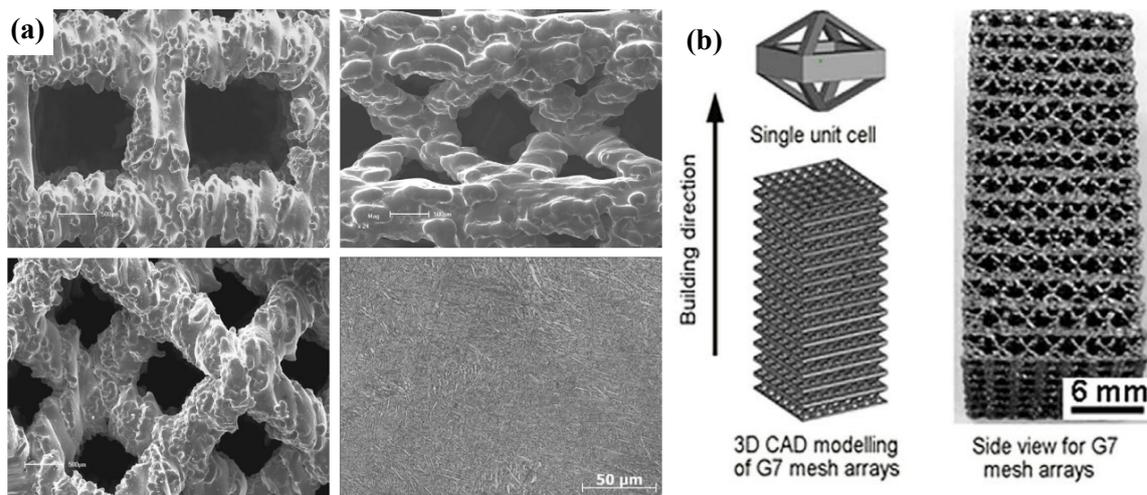
**Figure 11.** (a) The microstructures of Ti-6Al-4V porous samples with electron beam melting. (b) Porous structure model and side view of the Ti-24Nb-4Zr-8Sn component processed via electron beam melting [71]. (Reused with permission from ref. [71]. Copyright 2017, WILEY-VCH Verlag GmbH & Co. KGaA).
