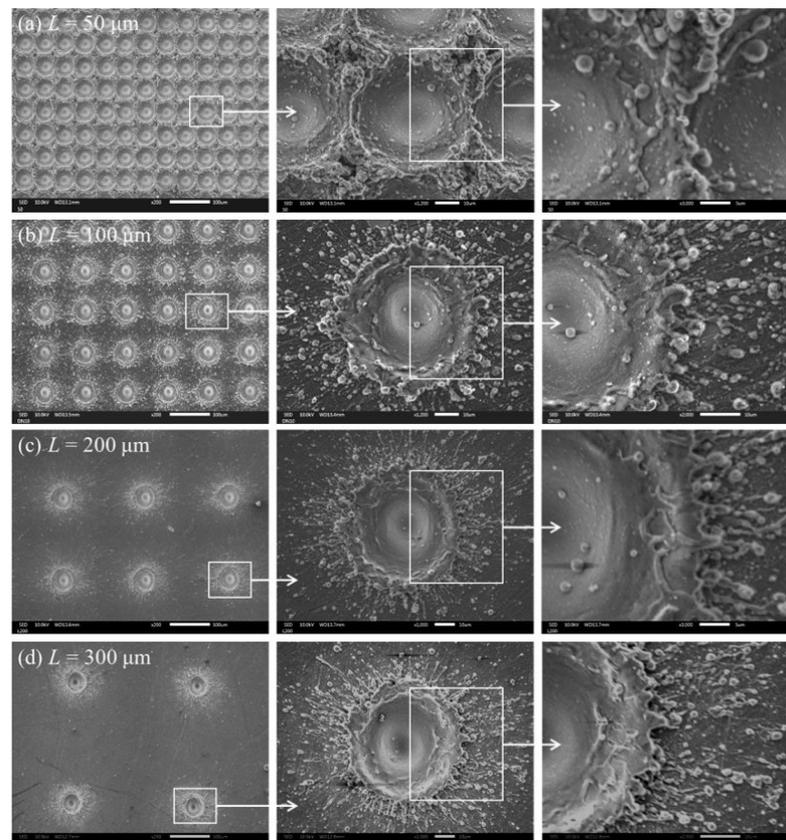
**Figure 9.** SEM images of the pitted surfaces of  $N = 10$  processed with different scanning spaces. (a)  $L = 50 \mu\text{m}$ ; (b)  $L = 100 \mu\text{m}$ ; (c)  $L = 200 \mu\text{m}$ ; (d)  $L = 300 \mu\text{m}$ . [63]. (Reused with permission from ref. [63]. Copyright 2021, Elsevier).
