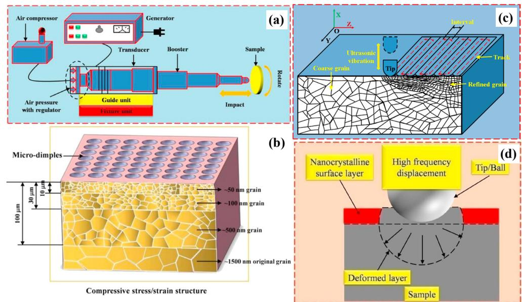
**Figure 6.** (a) Experimental installation diagram of the UNSM technique; (b) schematic of the microstructure of the modified layer under UNSM; (c) schematic diagram of UNSM; (d) schematic diagram of continuous UNSM processing. [46]. (Reused with permission from ref. [46]. Copyright 2021, Elsevier).
