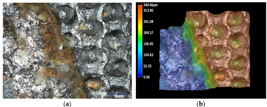
**Figure 4.** Images of anilox dot graticule area (a) Visible example of (I) damage to inkpot thresholds; (b) 3D microscopy image.
