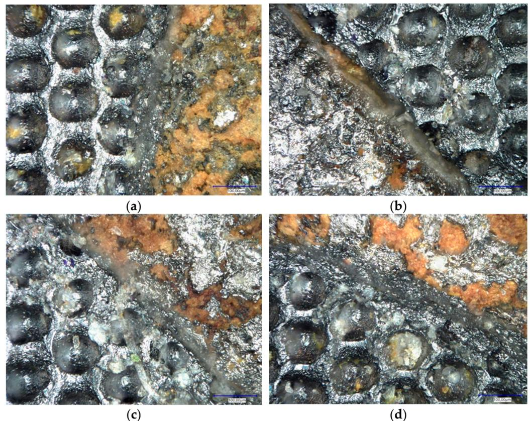
**Figure 5.** Various types of permanent damage to the ceramic coating of an anilox roll: (a) Example of (II) damage; (b) Example of (III) damage; (c) Example of (IV) damage; (d) Example of (V) damage.
