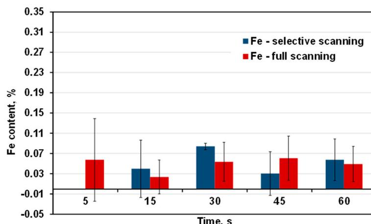
**Figure 2.** Concentrations of Fe as a function of scanning time determined using portable XRF analyser in selective and full mode.
