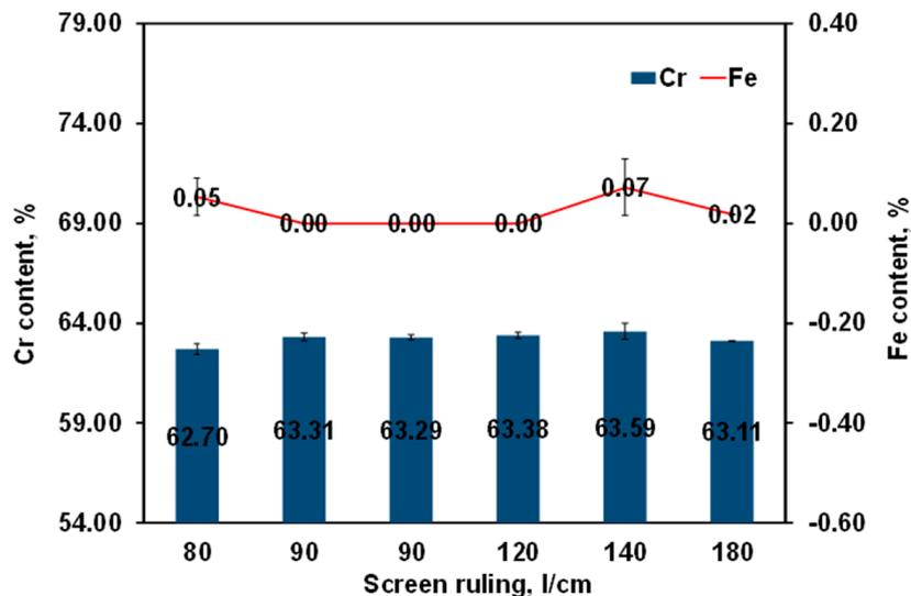
Figure 3. Concentrations of Cr and Fe as a function of screen ruling determined using a portable XRF analyser.
