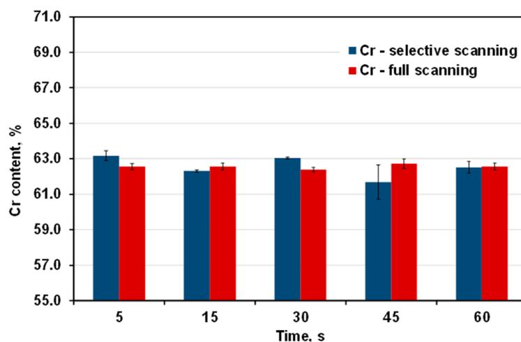
Figure 1. Concentrations of Cr as a function of scanning time determined using portable XRF analyser in selective and full mode.
