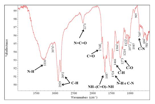
Figure 2. FTIR spectrum in the diffuse reflectance modality of the polyurethane product.
