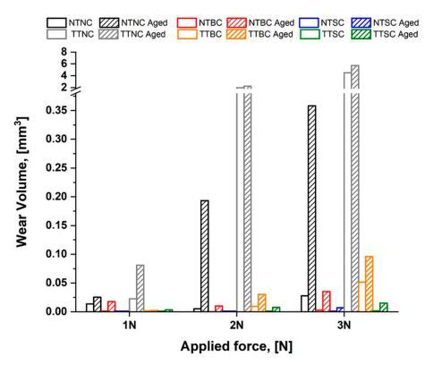
**Figure 8.** Wear volume average values for untreated (NT) and thermally treated (TT) samples, which were uncoated (NC) and coated with the polyurethane product via either brushing (BC) or spraying (SC), before and after 168 h of artificial ageing in Solar Box.
