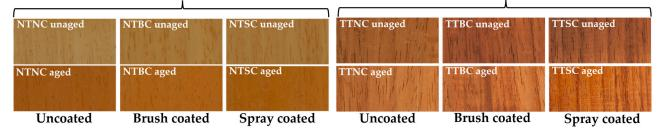
**Figure 1.** Photographs of specimen details for each typology: untreated without coating (NTNC); untreated and coated via brushing (NTBC); untreated and coated via spraying (NTSC); thermally treated without coating (TTNC); thermally treated and coated via brushing (TTBC); and thermally treated and coated via spraying (TTSC).
