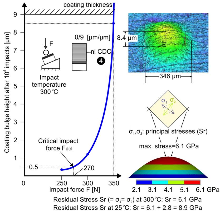
**Figure 6.** Determination of critical force  $F_{del}$  for coating delamination and coating residual stresses considering the bulge dimensions formed during the inclined impact test.
