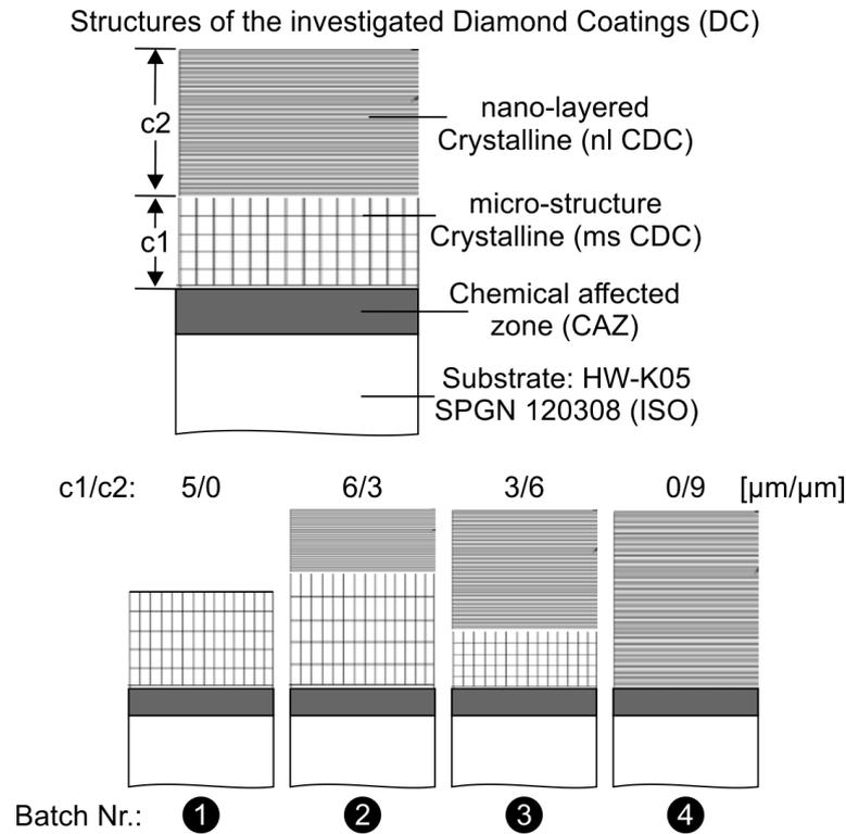
**Figure 1.** The employed cemented carbide insert batches with various coating architectures.
