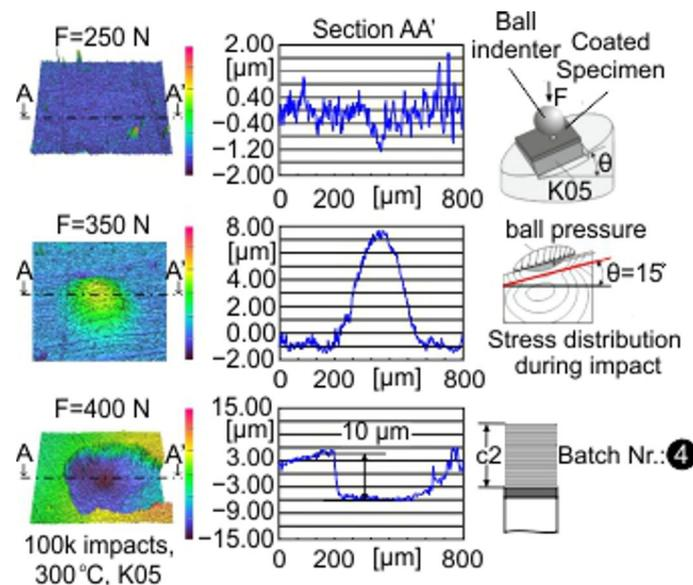
**Figure 5.** Formation of a coating bulge due to interface fatigue failure during the inclined impact test in the examined case of the 4th batch.
