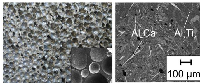
Workpiece material: Aluminium foam
