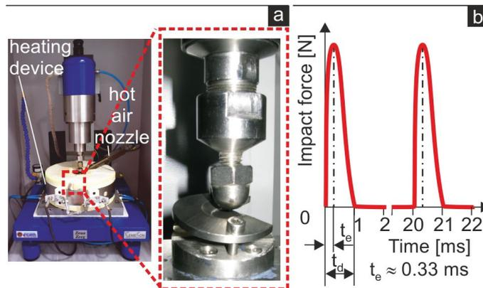
**Figure 2.** (a) The device used to conduct inclined impact tests; (b) the applied force signals.
