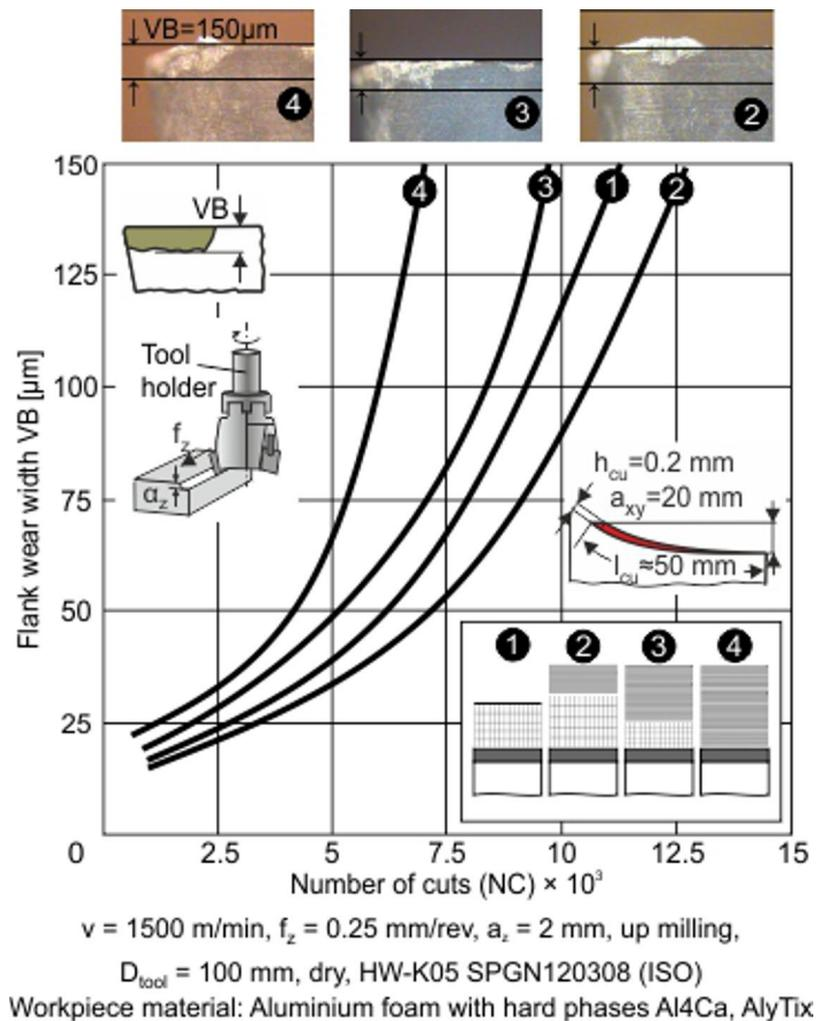
**Figure 9.** Flank wear width VB over the number of cuts in milling for the investigated CDCs with various structure architectures.
