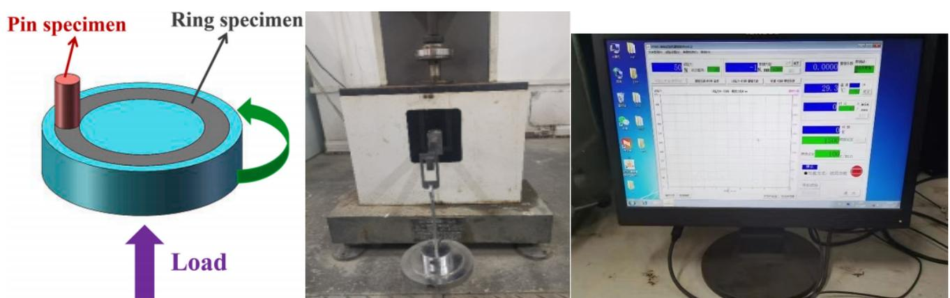
**Figure 1.** Pin disc friction and wear experimental device.
