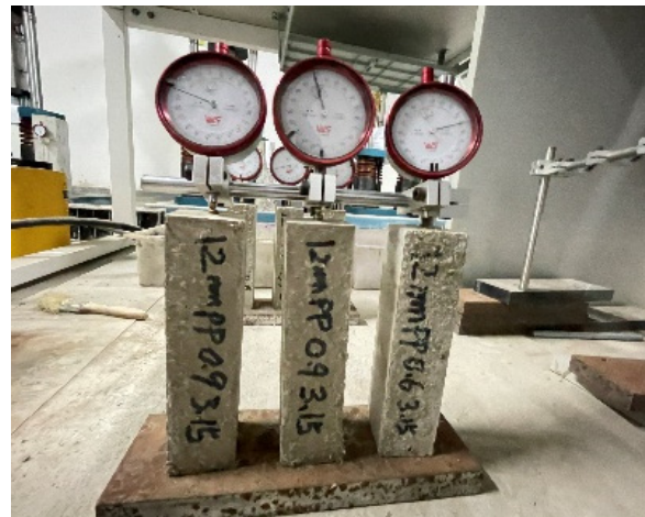
Figure 2. The measurement of the dry shrinkage rate.
