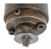
Figure 3. UFSP tool: concave shoulder with triflute left-hand threaded conical pin.
