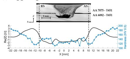
**Figure 11.** Eddy currents and microhardness profiles along the X direction of the plates reinforced with SiC particles: (a) AA7\_6\_1120/180\_P and (b) AA7\_6\_900\_180\_P.
