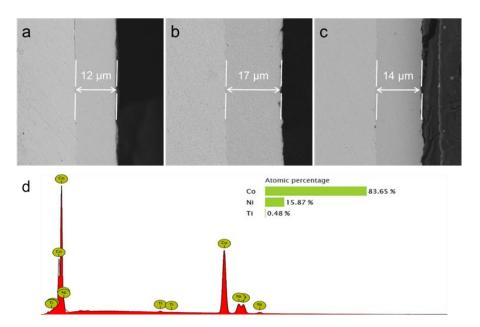
**Figure 6.** Cross-section of Co–Ni–TiO<sub>2</sub> films prepared with different content of TiO<sub>2</sub> sol: (**a**) 0 mL/L; (**b**) 12.5 mL/L; (**c**) 50 mL/L, and (**d**) the EDS results of the Co–Ni–12.5 mL/L TiO<sub>2</sub> sample.
