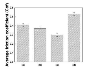
**Figure 8.** The friction coefficient of  $Co-Ni-TiO_2$  films prepared with diverse content of  $TiO_2$  sol: (a) 0 mL/L; (b) 5 mL/L; (c) 12.5 mL/L; (d) 50 mL/L.
