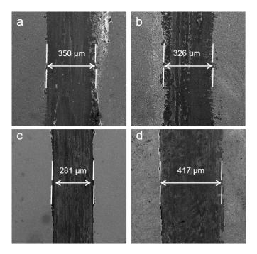
Figure 9. Wear track of Co $-Ni-TiO_2$  films prepared with different concentrations of TiO<sub>2</sub> sol: (a) 0 mL/L; (b) 5 mL/L; (c) 12.5 mL/L; (d) 50 mL/L.
