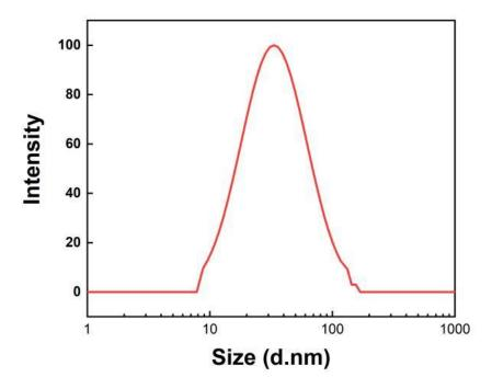
Figure 3. Size distribution of TiO<sub>2</sub> nanoparticles generated by adding sol into DI water.
