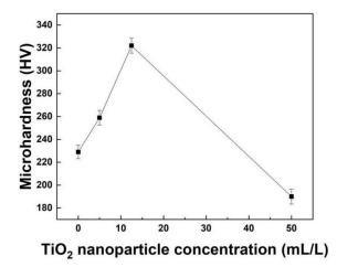
Figure 7. Microhardness tested on Co-Ni-TiO<sub>2</sub> films with diverse TiO<sub>2</sub> sol content.
