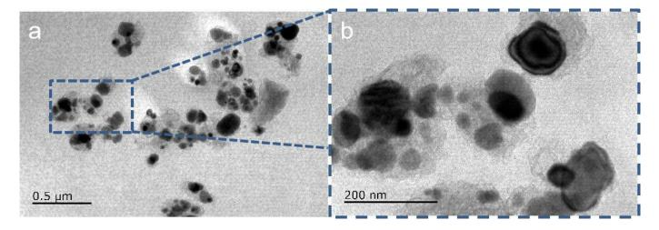
**Figure 1.** TEM images were taken on the generated TiO<sub>2</sub> nanoparticles made by adding sol into DI water. (**a**) TEM image, (**b**) Enlarged image for nanoparticles.
