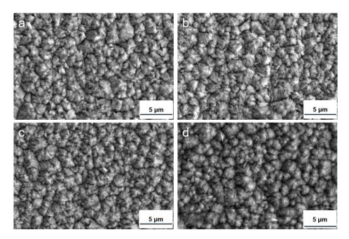
**Figure 4.** Surface morphology of Co–Ni–TiO<sub>2</sub> films prepared with different content of TiO<sub>2</sub> sol: (**a**) 0 mL/L; (**b**) 5 mL/L; (**c**) 12.5 mL/L; (**d**) 50 mL/L.
