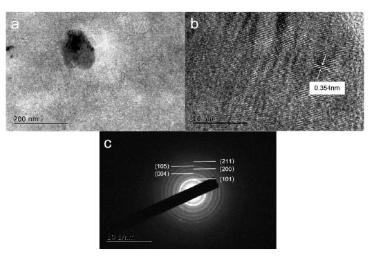
**Figure 2.** The microstructure of a single TiO<sub>2</sub> nanoparticle. (**a**) TEM image, (**b**) HR–TEM micrograph, (**c**) electron diffraction pattern.
