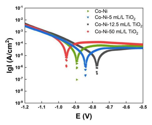
Figure 10. Potentiodynamic polarization curves of different Co-Ni-TiO<sub>2</sub> films.
