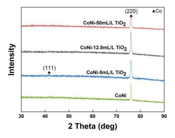
Figure 5. X-ray diffractograms recorded on the prepared Co-Ni-TiO<sub>2</sub> films.
