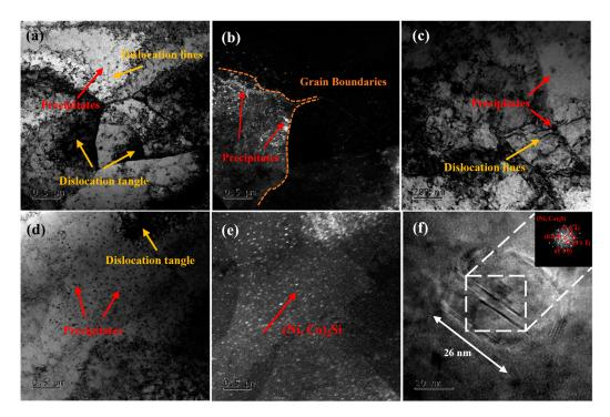
**Figure 3.** TEM and HRTEM images of the new type of Cu-1.1–Ni-0.7–Co-0.45–Si-0.3Cr alloy deformed at 600 °C and 0.01 s<sup>-1</sup>. (a) Bright-field TEM image, (b) dark-field TEM image of (a), (c) bright-field TEM image, (d) bright-field TEM image of precipitates, (e) dark-field TEM image of precipitates, (f) HRTEM image and corresponding FFT pattern of a (Ni, Co)<sub>2</sub>Si particle.
