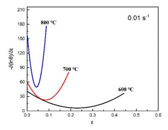
**Figure 9.** Strain hardening rate  $-\partial(\ln\theta)/\partial\epsilon$ - $\epsilon$  curve of the new type of Cu-1.1–Ni-0.7–Co-0.45–Si-0.3Cr alloy at different deformation temperatures.
