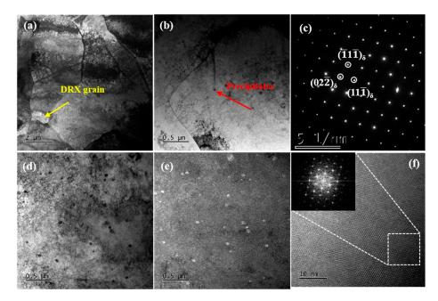
**Figure 5.** TEM and HRTEM images of the new type of Cu-1.1–Ni-0.7–Co-0.45–Si-0.3Cr alloy deformed at 800 °C and  $0.01 \, \rm s^{-1}$ . (**a**,**b**) Bright-field TEM image, (**c**) SAED analysis of precipitates in B, (**d**) bright-field TEM image, (**e**) dark-field TEM image of (**d**), (**f**) HRTEM image and corresponding FFT pattern of a (Ni, Co)<sub>2</sub>Si particle.
