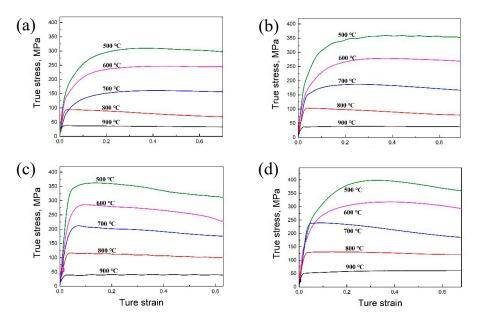
**Figure 1.** Flow stress–strain curves of the new type of Cu-1.1–Ni-0.7–Co-0.45–Si-0.3Cr alloy at different compression temperatures with different strain rates: (a)  $0.001 \, \mathrm{s}^{-1}$ , (b)  $0.01 \, \mathrm{s}^{-1}$ , (c)  $0.1 \, \mathrm{s}^{-1}$ , (d)  $1 \, \mathrm{s}^{-1}$ .
