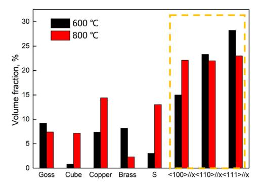
**Figure 12.** Texture composition of the new type of Cu-1.1–Ni-0.7–Co-0.45–Si-0.3Cr alloy at deformation temperatures of 600  $^{\circ}$ C and 800  $^{\circ}$ C.
