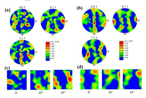
**Figure 11.** Pole figure and ODF maps of the new type of Cu-1.1–Ni-0.7–Co-0.45–Si-0.3Cr alloy in different deformation states: (**a**,**c**)  $600 \,^{\circ}$ C and  $0.01 \, \text{s}^{-1}$ , (**b**,**d**)  $800 \,^{\circ}$ C and  $0.01 \, \text{s}^{-1}$ .
