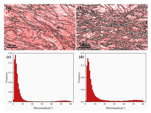
**Figure 8.** Orientation maps and misorientation angle distributions of the new type of Cu-1.1–Ni-0.7–Co-0.45–Si-0.3Cr alloy in different deformation states: (**a,c**) 600  $^{\circ}$ C and 0.01 s<sup>-1</sup>, (**b,d**) 800  $^{\circ}$ C and 0.01 s<sup>-1</sup>.
