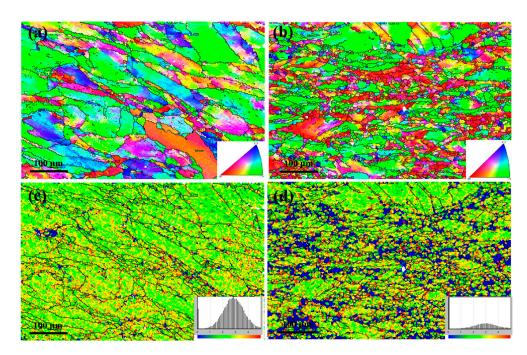
**Figure 7.** EBSD-IPF and corresponding KAM maps of the new type of Cu-1.1–Ni-0.7–Co-0.45–Si-0.3Cr alloy in different deformation states: (**a**,**c**) 600  $^{\circ}$ C and 0.01 s<sup>-1</sup>, (**b**,**d**) 800  $^{\circ}$ C and 0.01 s<sup>-1</sup>.
