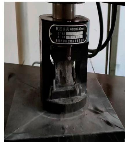
**Crushed specimens****Figure 2.** The measuring process of flexural and compressive strengths.
