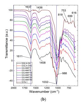
**Figure 1.** ATR-FTIR spectra of gellan gum electrolytes, gellan gum/Na+SYN-1 nanocomposites, and Na+SYN-1 clay in the range of 4000 to 550 cm<sup>-1</sup> (a) and 2000 to 550 cm<sup>-1</sup> (b).
