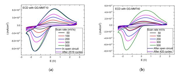
Figure 4. Voltammograms of the  $WO_3$ -ECDs with GG-MMT10 (a) and GG-MMT40 (b), measured from -2.8 to 2.5 V at 50, 100, 200, 300, and 500 mV/s after 2519 (a) and 420 (b) coloration/discoloration cycles.
