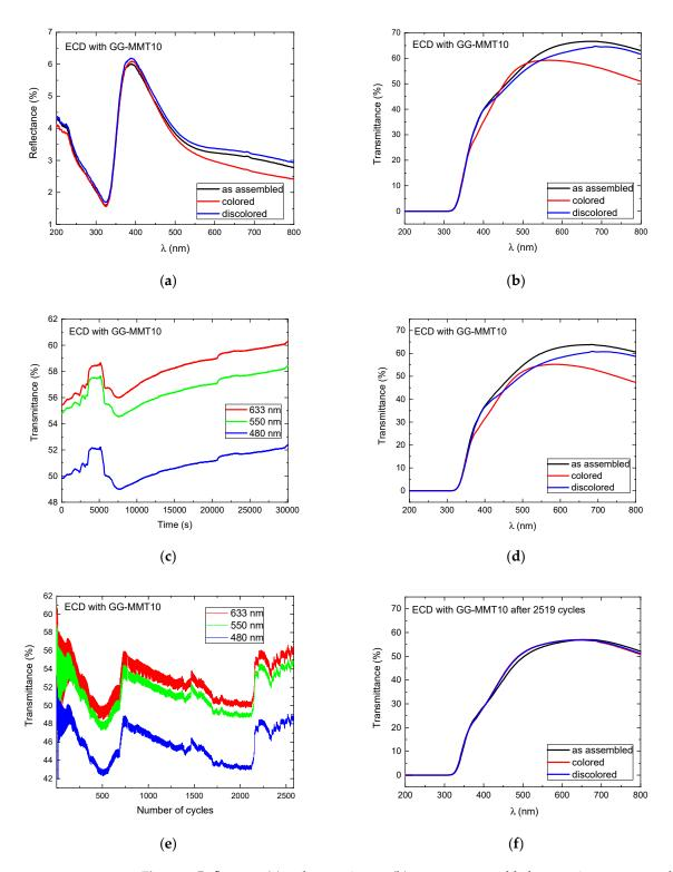
**Figure 6.** Reflectance (**a**) and transmittance (**b**) spectra as assembled; transmittance spectra during the open circuit at 480, 550, and 633 nm (**c**); transmittance spectra after the open circuit (**d**); transmittance spectra during the application of 2519 coloring/discoloring cycles at 480, 550, and 633 nm (**e**); and transmittance spectra after 2519 coloring/discoloring cycles (**f**) of WO<sub>3</sub>-ECD with GG-MMT10.
