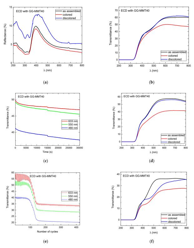
**Figure 7.** Reflectance (**a**) and transmittance (**b**) spectra of WO<sub>3</sub>-ECD with GG-MMT40 before the open circuit; transmittance spectra during the open circuit at 480, 550, and 633 nm (**c**); transmittance spectra after the open circuit (**d**); transmittance spectra during the application of 420 coloring/discoloring cycles at 480, 550, and 633 nm (**e**); and transmittance spectra after 420 coloring/discoloring cycles (**f**).
