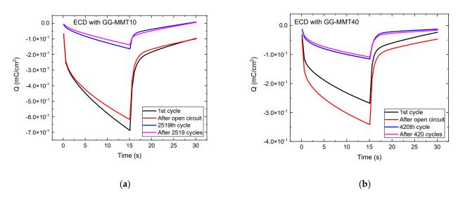
Figure 5. Charge density versus time for WO<sub>3</sub>-ECDs containing GG-MMT10 (a) and GG-MMT40 (b).
