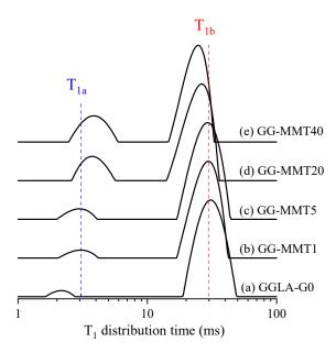
**Figure 2.** ILT spectra obtained from CWFP- $T_1$  signals for the films of GGLA-G0 (a), GG-MMT1 (b), GG-MMT5 (c), GG-MMT20 (d), and GG-MMT40 (e). The blue and red dashed lines are only a guide to identifying the  $T_{1a}$  and  $T_{1b}$  components, respectively.
