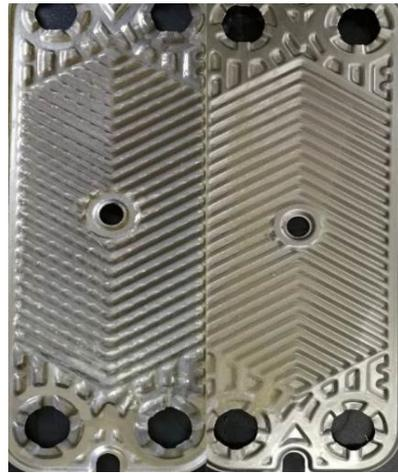
**Figure 11.** Macroscopic topography of the Ni–P–TiO<sub>2</sub> composite coating (**left**) and 316 stainless steel (**right**) at the MgO solution concentration is 400 mg/L.
