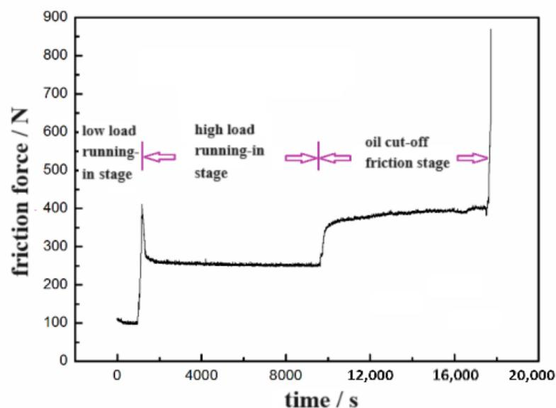
**Figure 4.** Trend in friction force variation in scuffing test.
