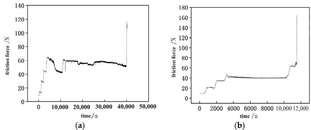
**Figure 9.** Friction force changes over time. (a) Cast-iron cylinder liner. (b) Al-Si alloy cylinder liner.
