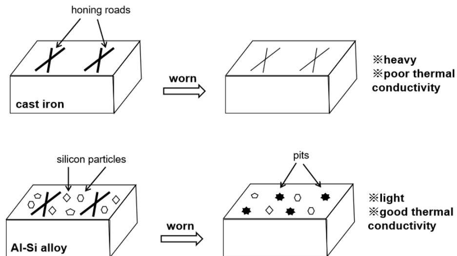
**Figure 13.** Schematic diagram of the cylinder liner wear process.
