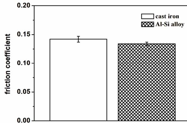
Figure 5. Friction coefficient of two matched pairs.
