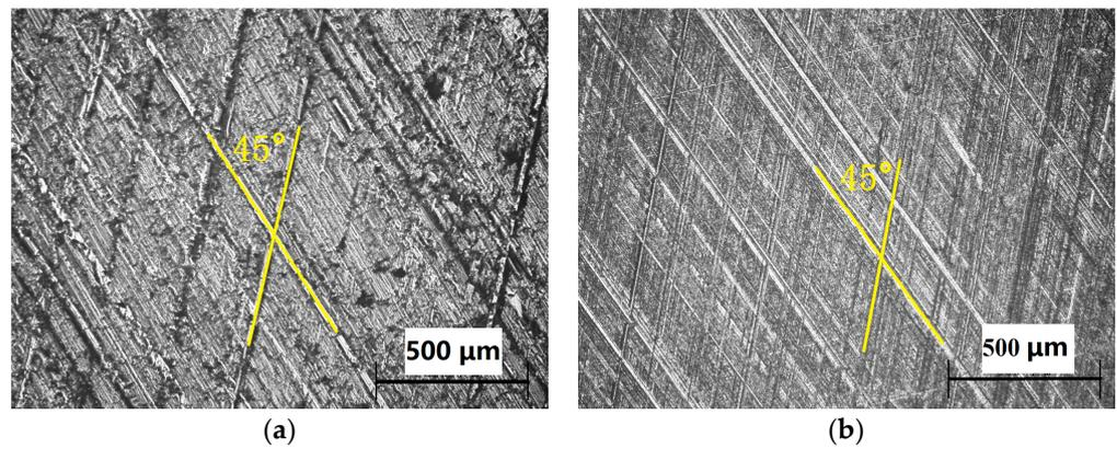
**Figure 1.** Honing roads on the surface of cylinder liners. (a) Cast-iron cylinder liner. (b) Al-Si alloy cylinder liner.
