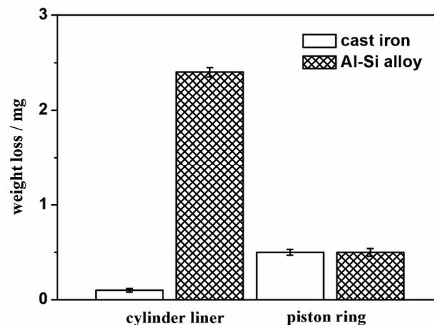
Figure 6. Weight loss of two matched pairs.
