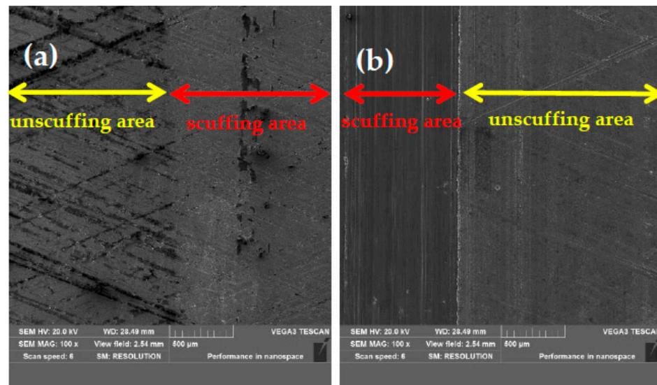
**Figure 11.** Scuffing surface morphology of cylinder liners: (a) cast-iron cylinder liner; (b) Al-Si alloy cylinder liner.
