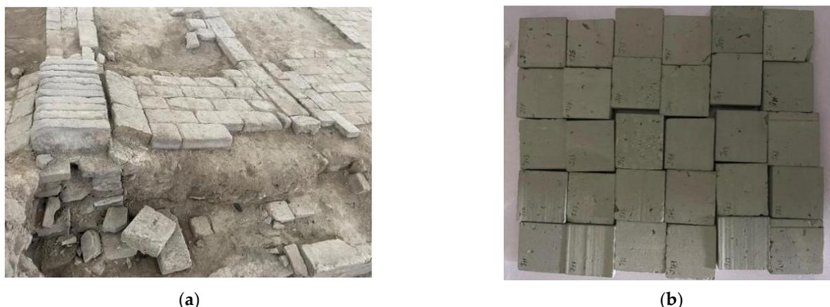
**Figure 3.** (a) Damaged bricks; (b) Small bricks to be coated.
