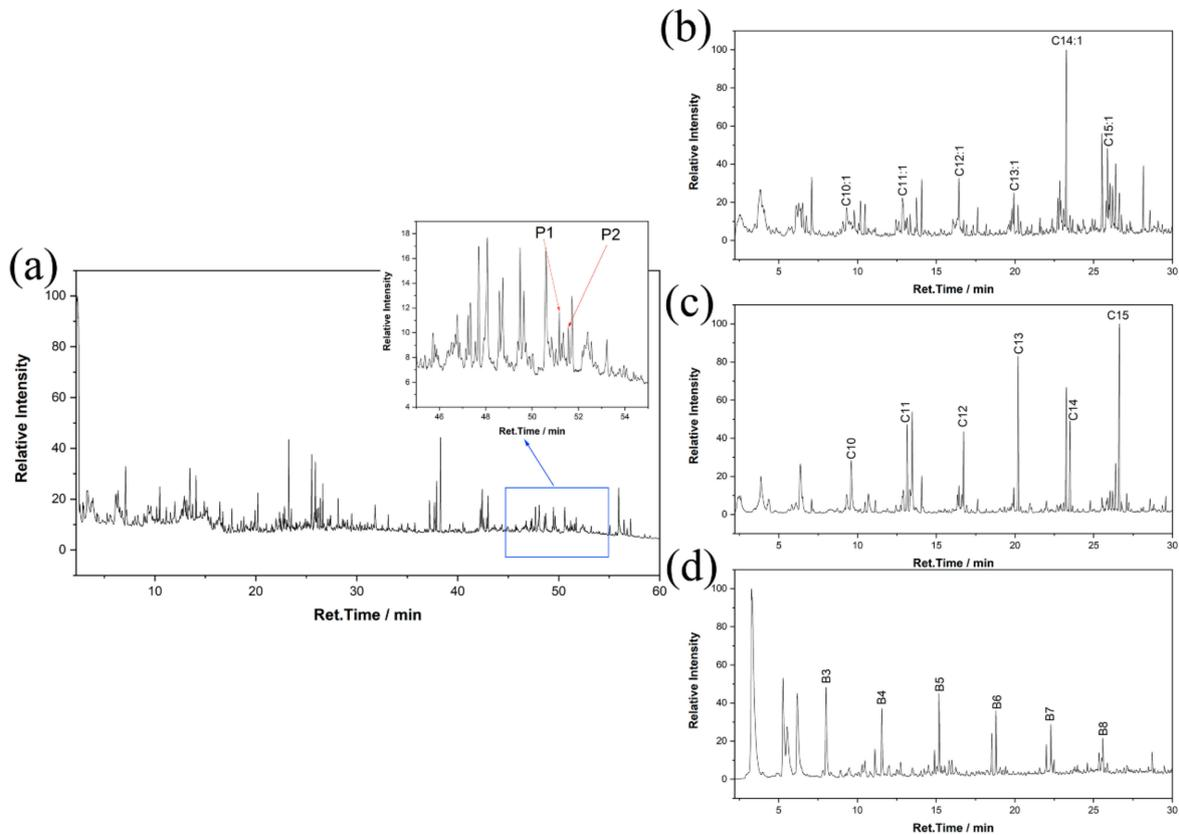
**Figure 4.** Chromatographic profiles obtained using THM-Py-GC/MS of red layer of sample 1: (a) total ion pyrogram; (b) m/z 55 extracted ion pyrogram; (c) m/z 57 extracted ion pyrogram; (d) m/z 91 extracted ion pyrogram.
