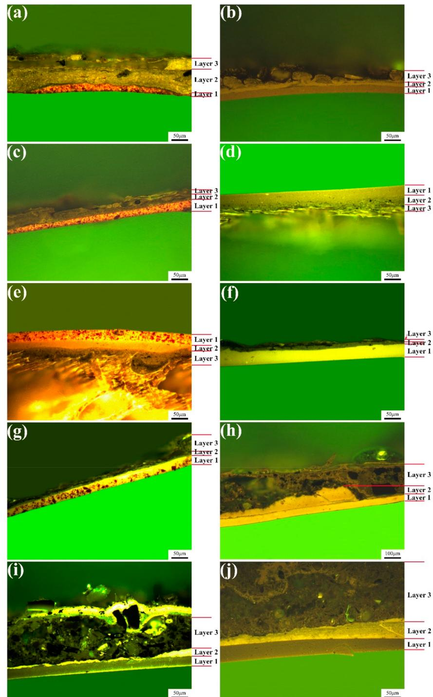
**Figure 2.** Cross-sectional photos of (a) Sample 1, (b) Sample 2 (black), (c) Sample 2 (red), (d) Sample 3 (black), (e) Sample 3 (red), (f) Sample 4 (black), (g) Sample 4 (red), (h) Sample 5, (i) Sample 6, and (j) Sample 7 under blue light.
