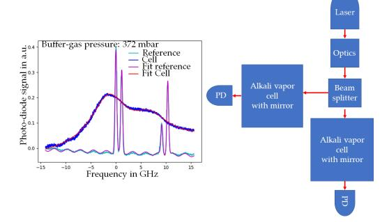
**Figure 6.** Left: Transmission spectrum of the passivated mirror cell for the evaluation of the buffer-gas pressure. Blue: measurement of the mirror cell; turquoise: measurement of a reference cell without mirror; red: calculated fit of the mirror cell; purple: calculated fit of the reference cell. The shift in the spectrum is calculated to determine the buffer-gas pressure. Right: Schematic setup of the reference measurement for the calculation of the buffer-gas pressure. PD: photodiode.
