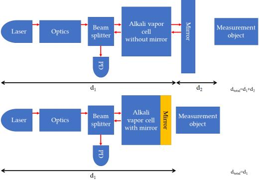
**Figure 1.** Schematic setup with an external mirror (**top**) and with an in-cell mirror (**bottom**). The distance between the measurement object and alkali vapor cell can be reduced significantly using the mirror inside the cell. PD: photodiode.
