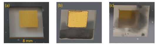
**Figure 3.** Photographs of fabricated cells. Cell (**a**) is the referec cell without decomposition, serving as a comparison for the other two. Cells (**b**,**c**) are shown after the steps of decomposition and annealing. Cell (**b**) has a passivation layer, while cell (**c**) does not. See the main text for more details.
