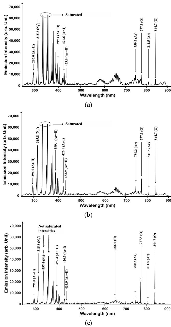
**Figure 4.** OES spectrum of N<sub>2</sub> + O<sub>2</sub> plasma: (a) the case of N<sub>2</sub> + O<sub>2</sub> (80:20), (b) the case of N<sub>2</sub> + O<sub>2</sub> (50:50), and (c) the case of N<sub>2</sub> + O<sub>2</sub> (20:80).
