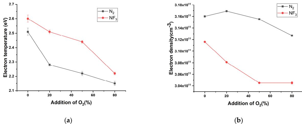
**Figure 9.** Plasma information of  $\text{N}_2$  and  $\text{NF}_3$  according to the amount of oxygen added: (a) electron temperature and (b) electron density.
