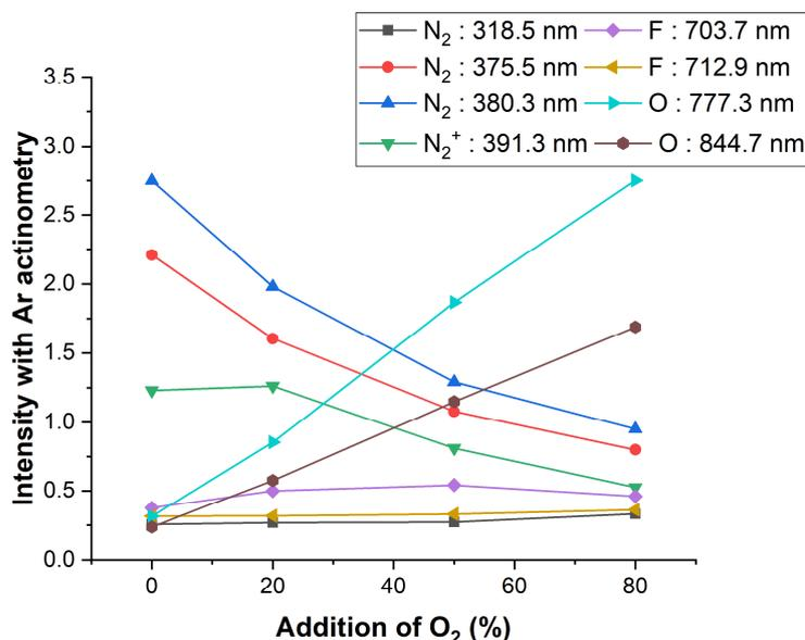
**Figure 8.** NF<sub>3</sub> + O<sub>2</sub> plasma peak intensity change with the addition of oxygen gas.
