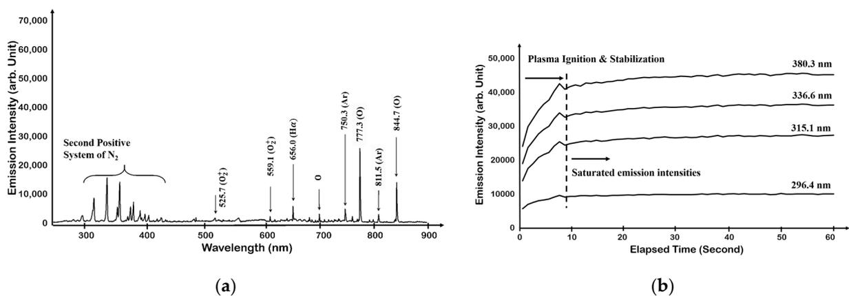
Figure 2. Optical emission spectrum of oxygen: (a) oxygen plasma and (b) change in  $O_2$  plasma intensity over time [27,28].
