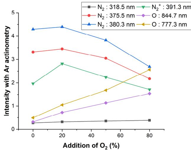
Figure 5. N<sub>2</sub> + O<sub>2</sub> plasma peak intensity change with the addition of O<sub>2</sub>.
