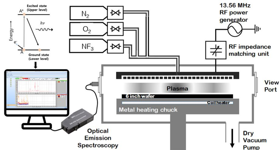
Figure 1. Experimental apparatus of a 13.56 MHz PECVD system with OES setup.
