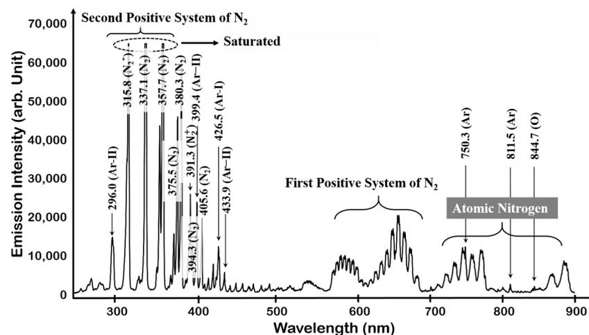
Figure 3. OES spectrum of N<sub>2</sub> plasm.
