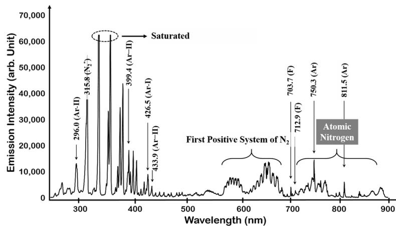
Figure 6. OES spectrum of NF<sub>3</sub> plasma.
