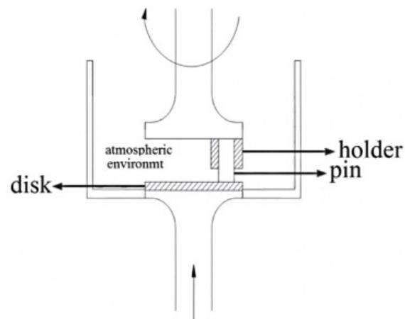
**Figure 3.** Schematic diagram of pin-disc friction and wear tester. Reprinted with permission from Ref. [11]. 2019, IOP Publishing Ltd.
