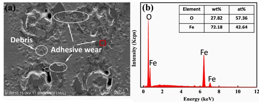
**Figure 10.** (a) SEM image of the wear scar and (b) EDS results of the sample. Adapted with permission from Ref. [71]. 2019, Elsevier.
