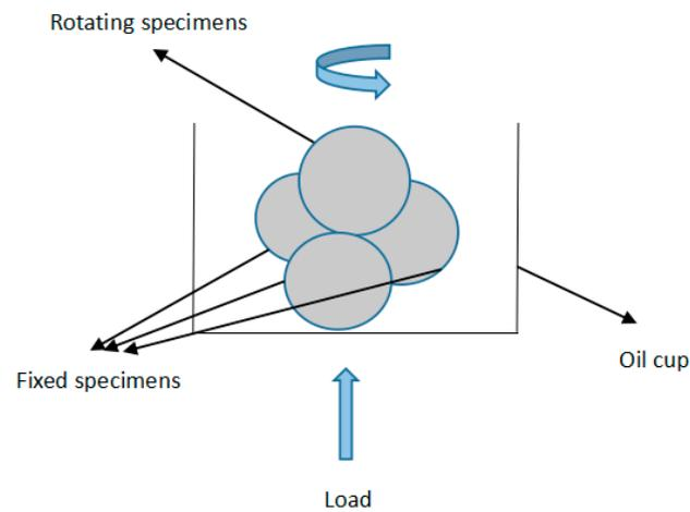
**Figure 2.** Schematic diagram of four-ball friction and wear tester.
