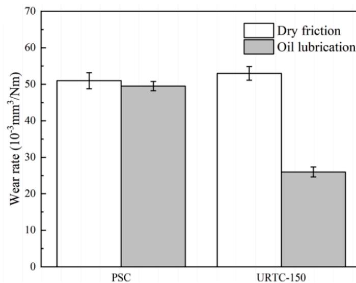
**Figure 6.** The wear rate of different materials under dry friction and oil lubrication. Reprinted with permission from Ref. [31]. 2021, Elsevier.
