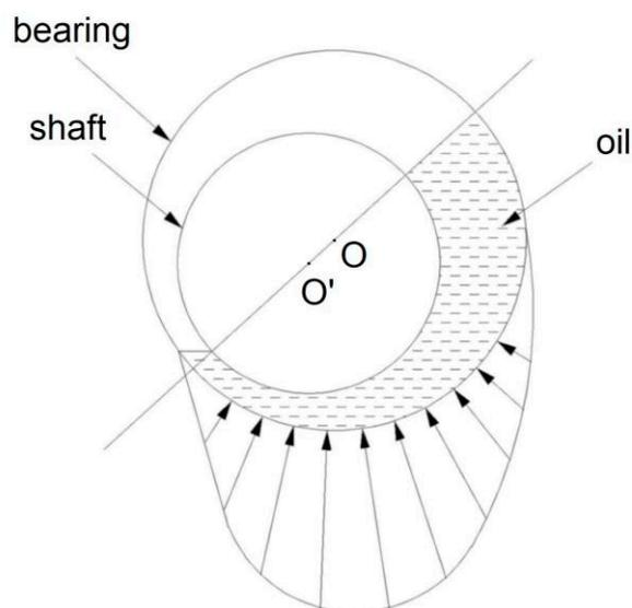
**Figure 1.** Schematic diagram of hydrodynamic lubrication.
