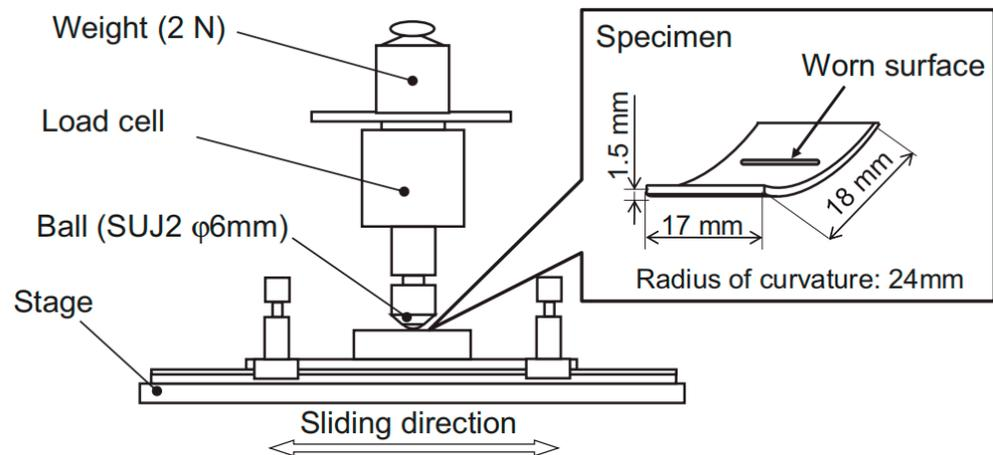
**Figure 5.** Schematic diagram of reciprocating friction and wear tester. Reprinted with permission from Ref. [13]. 2013, Elsevier.
