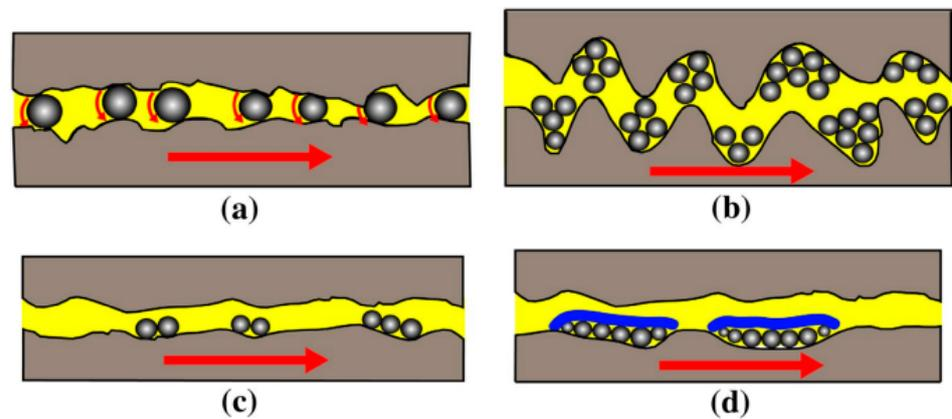
**Figure 7.** Schematic illustration of the (a) rolling mechanism; (b) self-repair, or mending mechanism; (c) polishing mechanism; and (d) tribo-film formation. Reprinted with permission from Ref. [33]. 2019, Springer.
