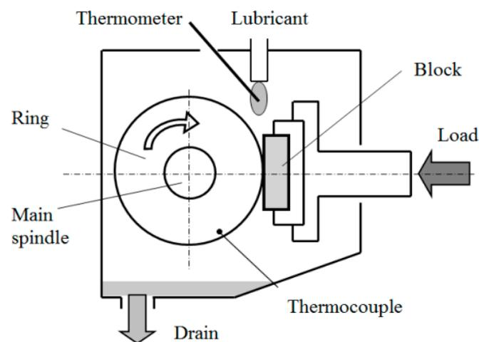
**Figure 4.** Schematic diagram of ring-block friction and wear tester. Reprinted with permission from Ref. [12]. 2017, The Japan Society of Mechanical Engineers.
