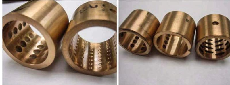
**Figure 9.** Surface textures of plain bearings. Reprinted with permission from Ref. [60]. 2007, Springer.
