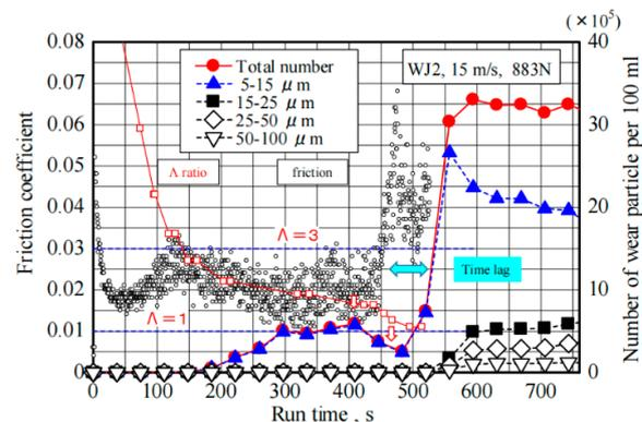
**Figure 11.** Relationships between the friction coefficient, number of wear particles, and run-time. Reprinted with permission from Ref. [74]. 2016, Japanese Society of Tribologists.
