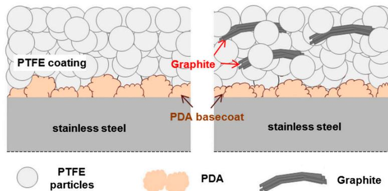
**Figure 8.** Schematic of PDA/PTFE and PDA/PTFE + graphite. Reprinted with permission from Ref. [49]. 2016, Springer.
