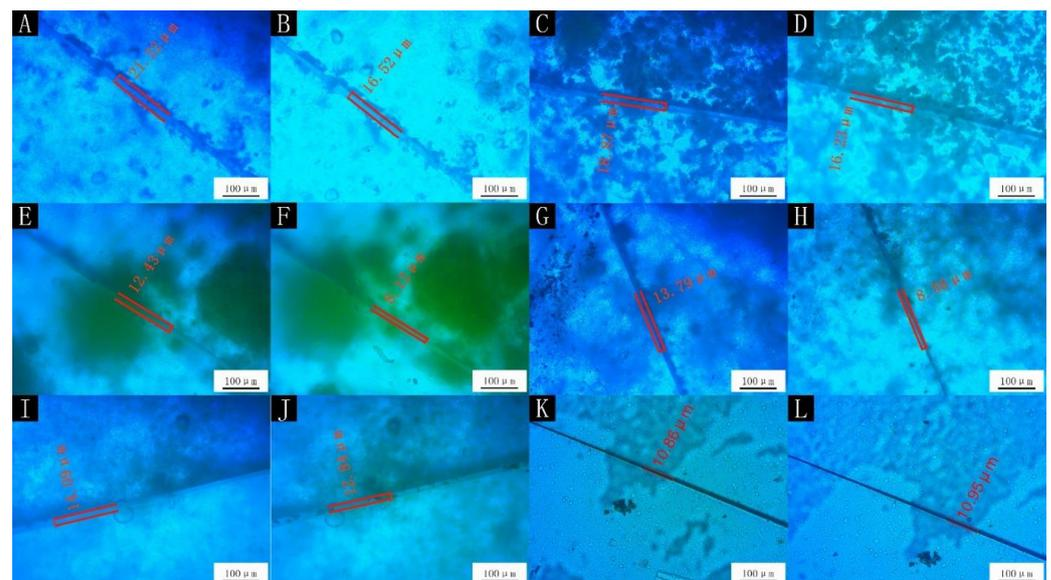
**Figure 10.** Micrographs of paint film self-healing test of five emulsifier microcapsules: (A) the first day of Span-80, (B) the fifth day of Span-80, (C) the first day of SDBS, (D) the fifth day of SDBS,
