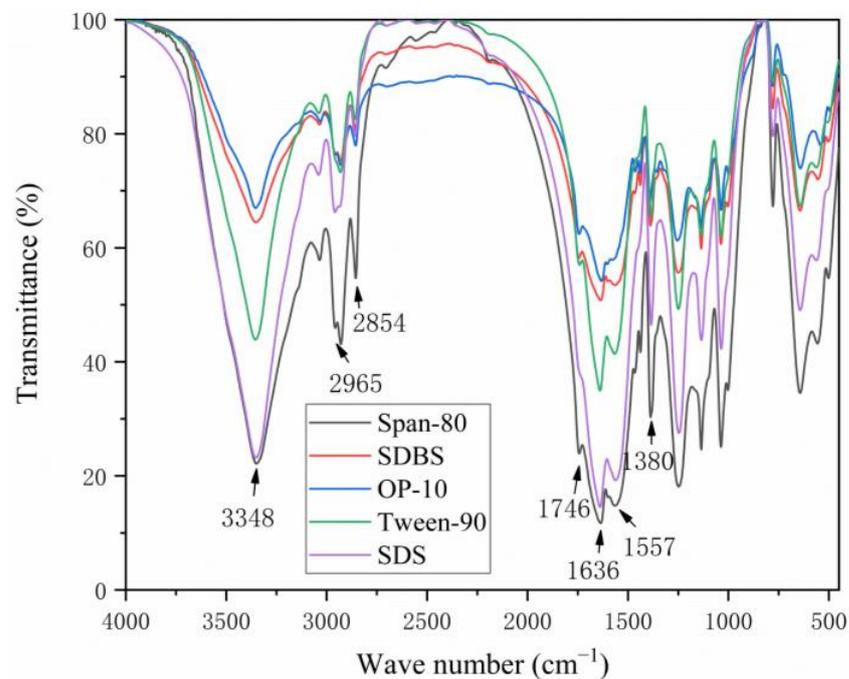
**Figure 4.** Infrared spectra of five emulsifier microcapsules.
