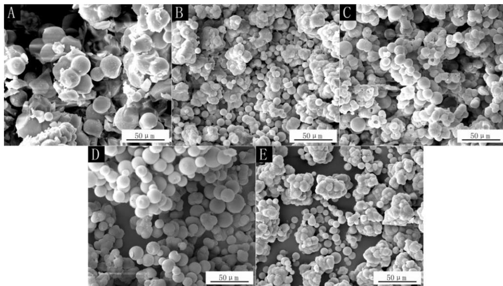
**Figure 2.** SEM of tung oil microcapsules emulsified by five emulsifiers (A) Span-80, (B) SDBS, (C) OP-10, (D) Tween-80, (E) SDS.
