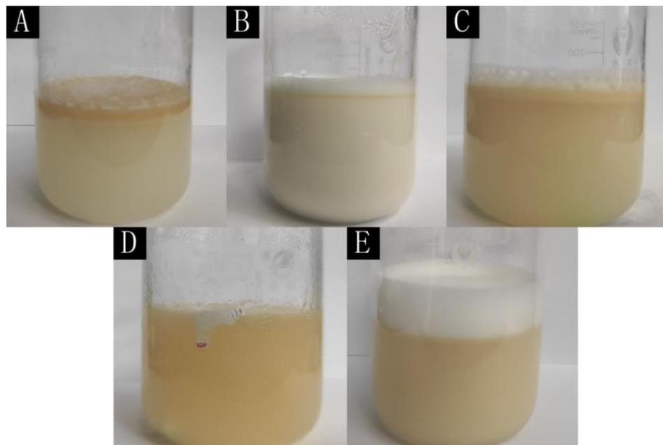
**Figure 1.** The core material emulsion emulsified by different emulsifiers: (A) Span-80, (B) SDBS, (C) OP-10, (D) Tween-80, (E) SDS.
