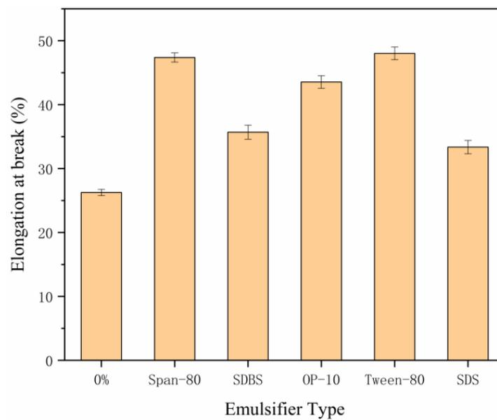
**Figure 6.** Effect of emulsifier on elongation at break of paint film.
