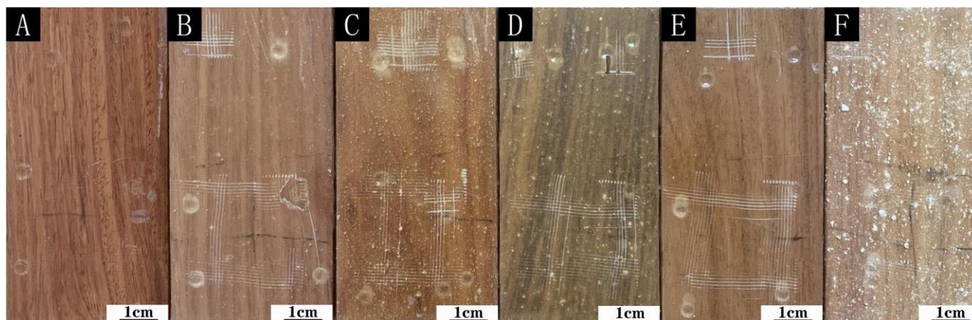
**Figure 5.** Morphology of paint film on the surface of basswood prepared with different emulsifiers (A) without microcapsules, (B) Span-80, (C) SDBS, (D) OP-10, (E) Tween-80, (F) SDS.
