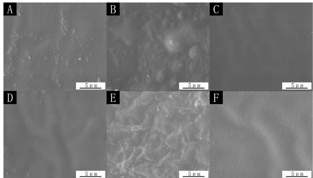
**Figure 9.** SEM of coating film: (A) Span-80, (B) SDBS, (C) OP-10, (D) Tween-80, (E) SDS, (F) no microcapsules.
