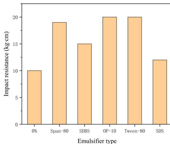
**Figure 7.** Effect of emulsifier on impact resistance of paint film.
