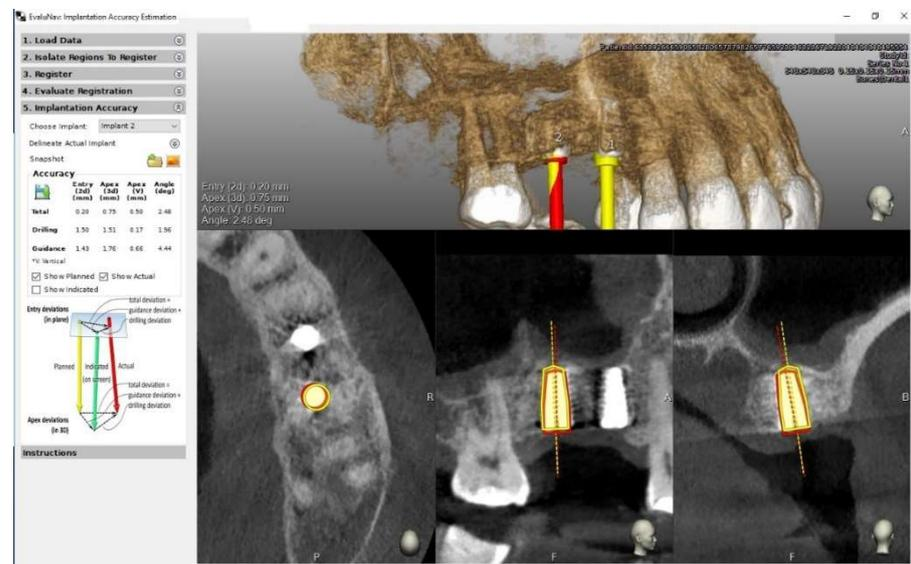
**Figure 5.** Comparison between planning (yellow) and actual implant position (red) based on preoperative and post-operative CBCT scans.
