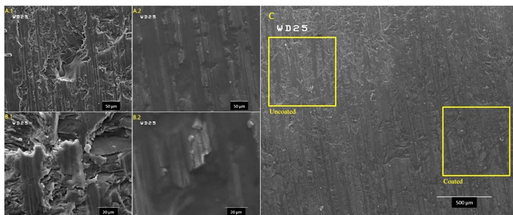
Figure 2. SEM images at 300\times (A) and 1000\times (B) magnifications comparing the bare (1) and coated (2) surfaces of a marble sample, primarily calcite, treated with formula 11. SEM image (C) of the transitional region between surfaces at 50\times magnification, the darker region has been coated.
