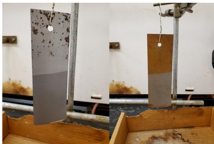
Figure 8. Stainless-steel sample before and after seven days of daily exposure to an oxidative rusting solution. The bottom half of the sample was dip coated.
