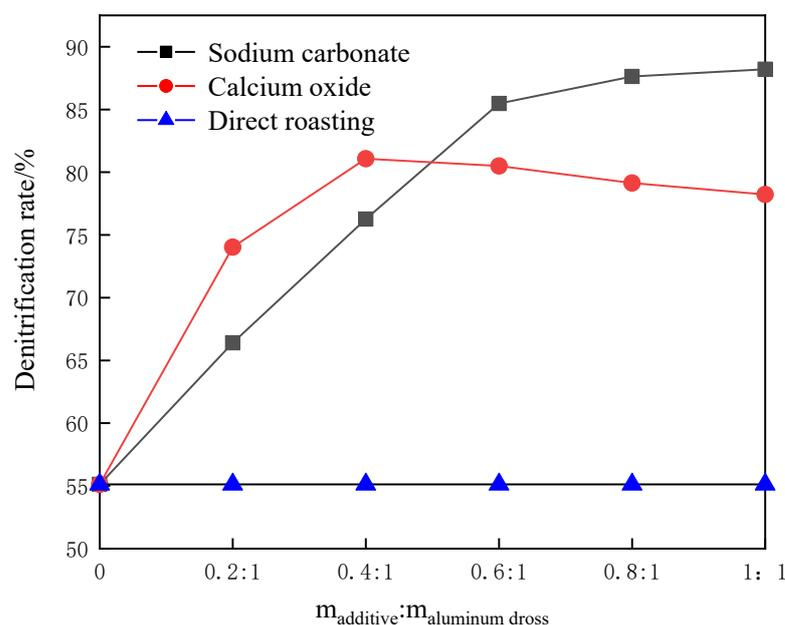
**Figure 4.** Denitrification rate of aluminum dross varies with mixture ratio.
