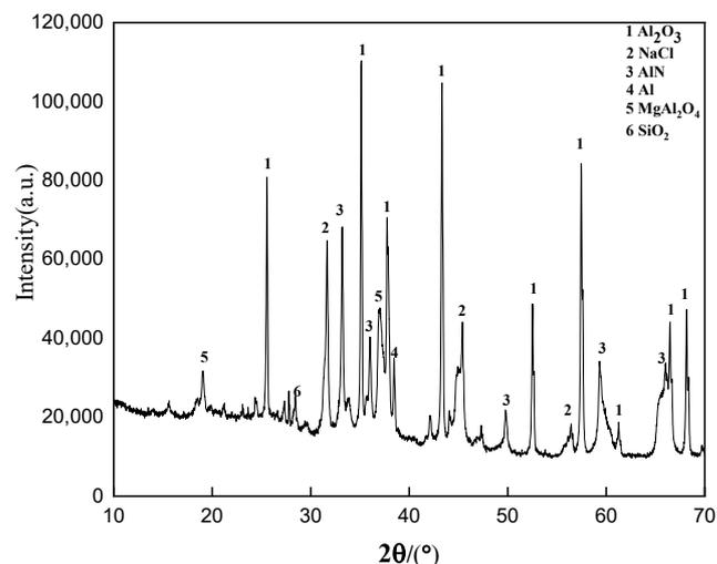
**Figure 2.** XRD pattern of original aluminum dross.
