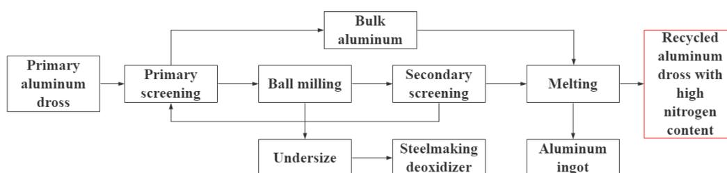
Figure 1. Production flow chart of aluminum dross.
