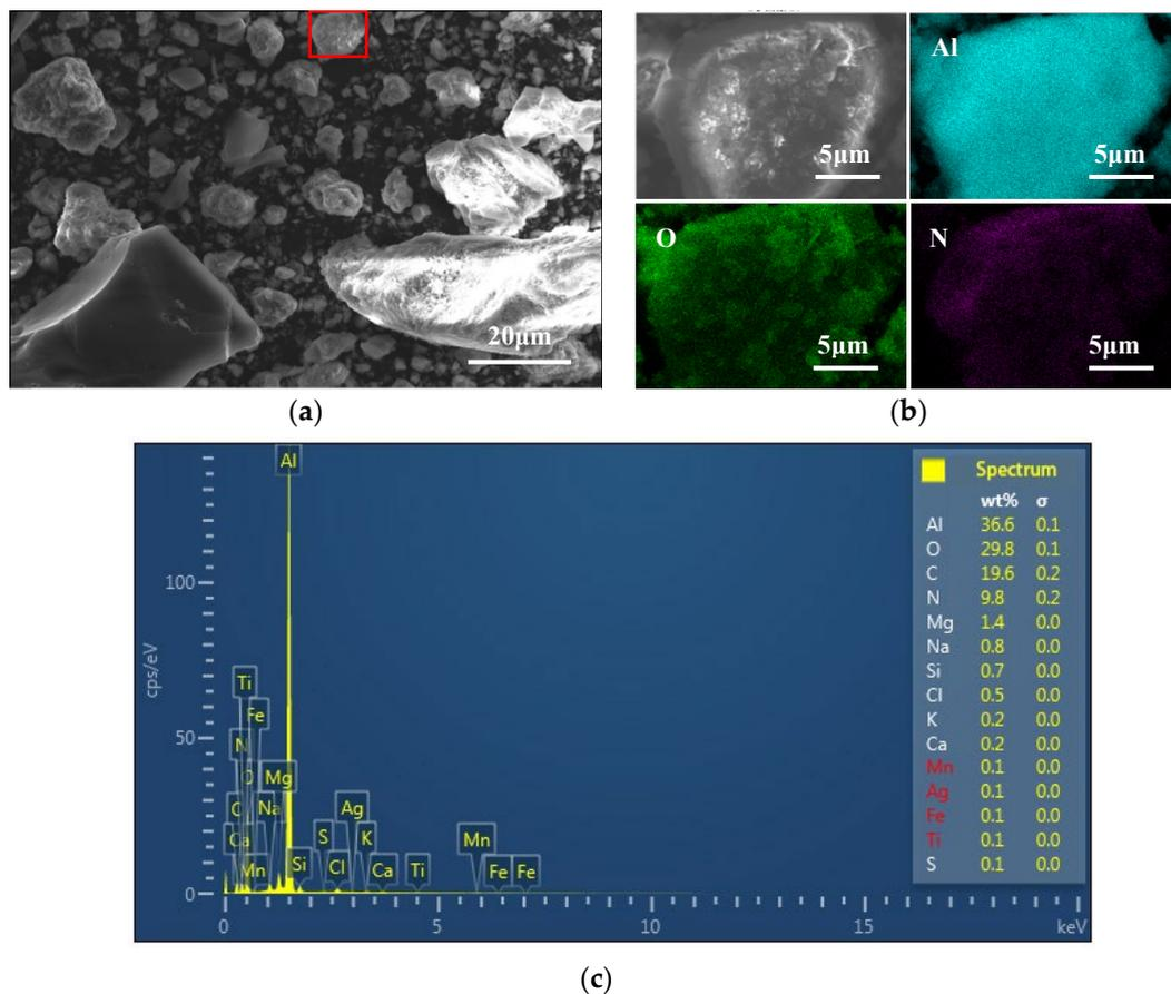
**Figure 3.** SEM-EDS image of original aluminum dross. (a) SEM of original aluminum dross; (b) SEM and micro-area element surface distribution of the red frame area; (c) EDS spectrum analysis of the red frame area.
