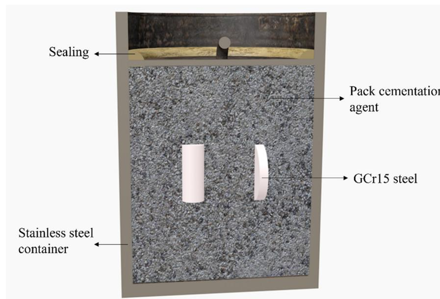
**Figure 2.** Vanadiumizing treatment schematic diagram.
