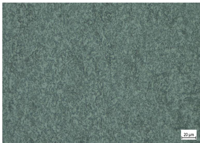
**Figure 1.** Microstructure of normalized GCr15 steel.
