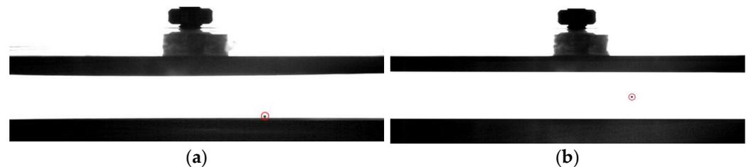
Figure 9. (a) The picture of the static particle (b) The picture of the lifting particle.
