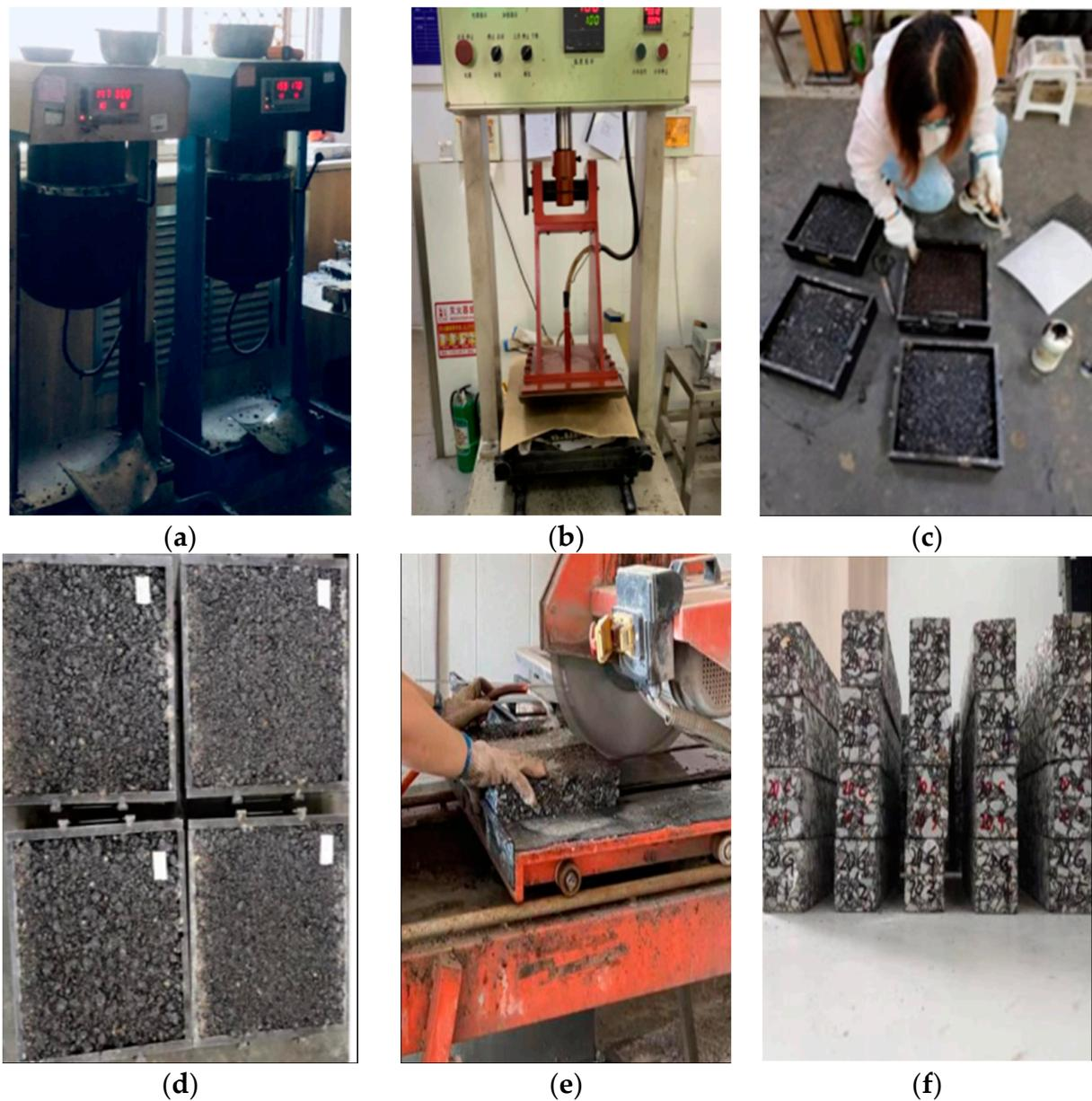
**Figure 1.** The preparation of test specimens. (a) Asphalt-mixture mixing; (b) layer rolling forming; (c) laying geosynthetics and brushing the tack coat; (d) double-layered asphalt slab; (e) plate cutting; (f) beam sample of the bending test.
