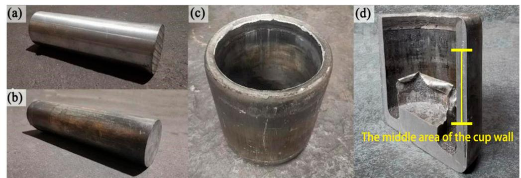
**Figure 2.** Schematic diagram of the formed part. (a) initial billet, (b) after upsetting and extrusion billet, (c) formed parts, and (d) the section of formed parts.
