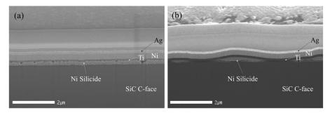
**Figure 3.** (a) RTA silicide ohmic contact and (b) laser silicide ohmic contact cross-sectional SEM images for the SiC C-face of Ni thicknesses of 100 nm in the fabricated JBS diodes.
