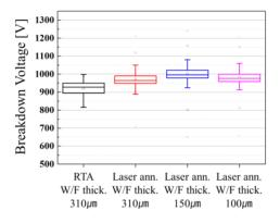
**Figure 5.** The breakdown voltage properties of fabricated JBS diodes at a current of  $250 \ \mu$ A in TO-220 packages.
