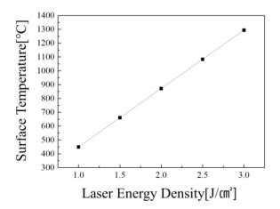
Figure 2. The surface temperature simulation of energy density (provided by SHI).
