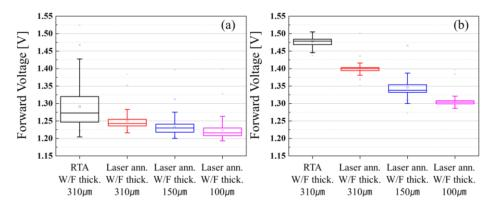
**Figure 4.** The forward bias properties of fabricated JBS diodes at (**a**) a current of 10 A on wafer die chips and (**b**) a current of 20 A on TO-220 packages.
