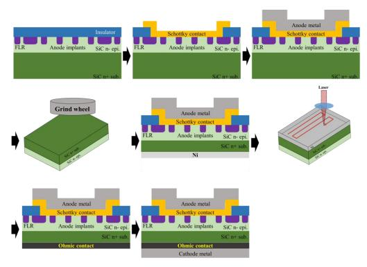
**Figure 1.** Schematic flow chart of the fabrication of a JBS diode with grinding and laser annealing processes.
