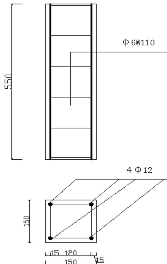
**Figure 4.** The structural dimension of the short column.
