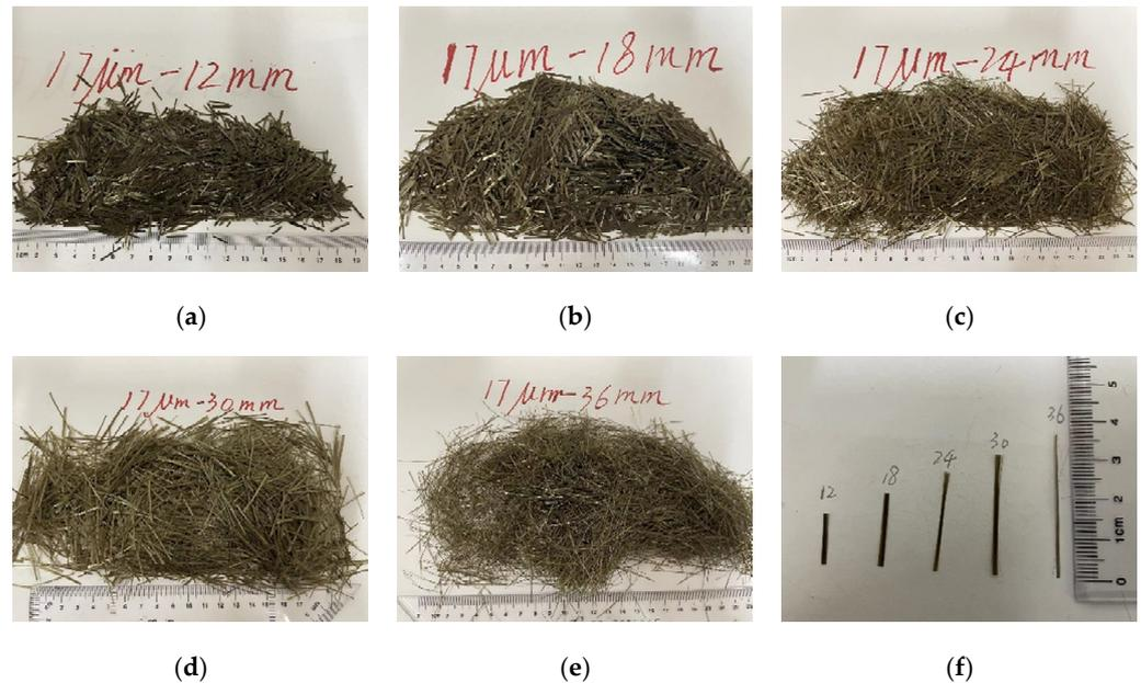
**Figure 1.** The five lengths of basalt fiber: (a)  $L = 12$  mm; (b)  $L = 18$  mm; (c)  $L = 24$  mm; (d)  $L = 30$  mm; and (e)  $L = 36$  mm; and (f) a schematic diagram of the different fiber lengths.**Table 2.** The physical and mechanical properties of the basalt fiber.
