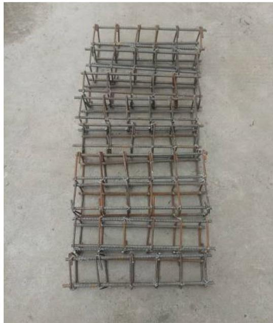
Figure 5. The reinforcement of the short column.
