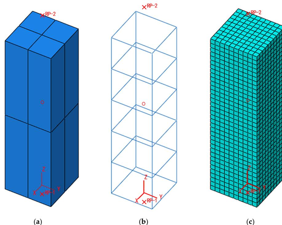
**Figure 10.** The finite element model of the short column: (a) the entity model; (b) the reinforcing element; and (c) the concrete unit.
