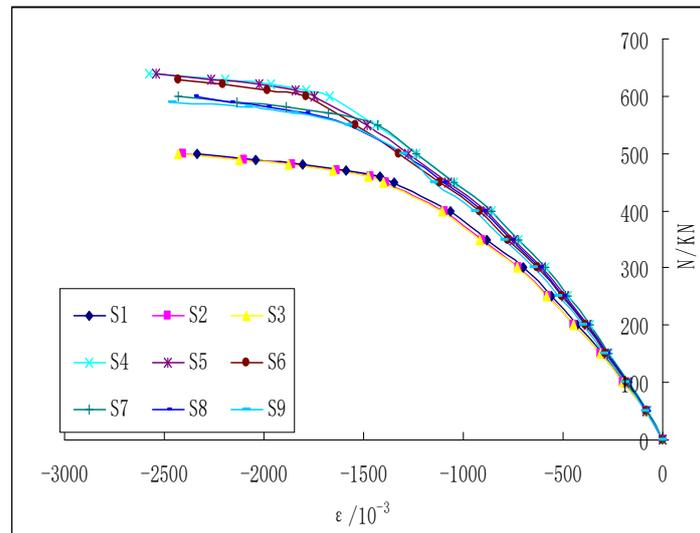
**Figure 8.** The average strain curve of the concrete.
