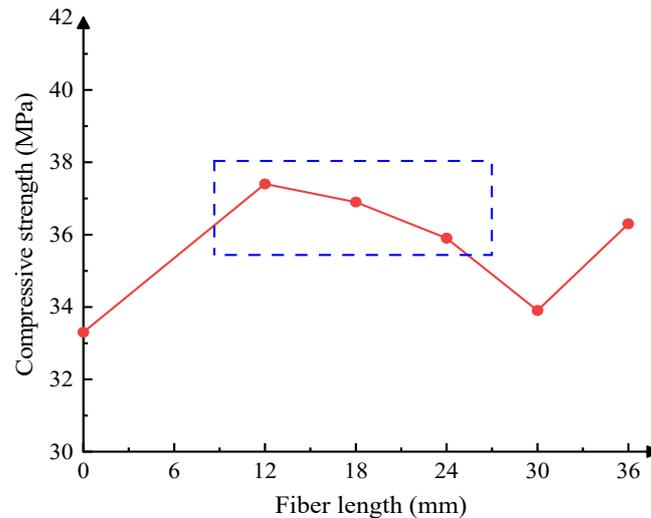
Figure 2. The 28 d compressive strength of the BRFC with different fiber lengths.
