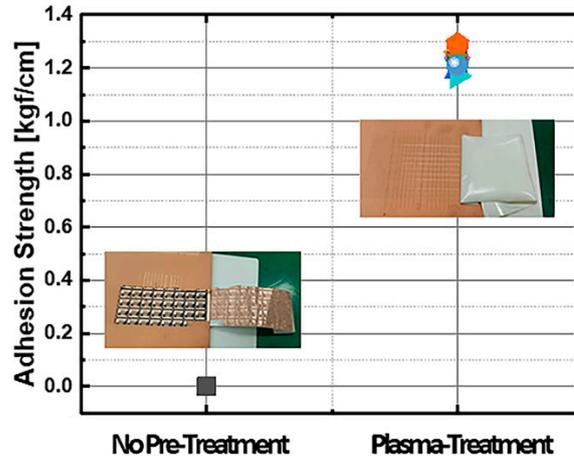
**Figure 9.** Effect of plasma treatment on adhesion strength between resin and Cu interface.
