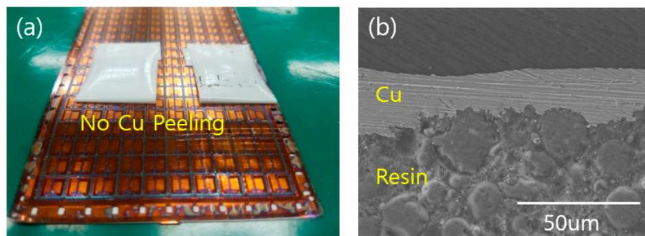
**Figure 10.** Moisture absorption evaluation of two-layer Rt-QFN: (a) Peel off tape test after moisture absorption; (b) SEM image of the interface between resin and Cu.
