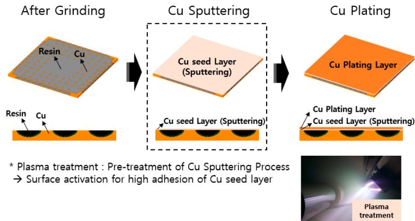
Figure 3. HDS Cu sputtering process w/plasma pretreatment to secure high adhesion.
