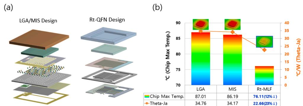
**Figure 11.** Comparison of heat dissipation performance between LGA and Rt-QFN substrate: (a) Structure of LGA/MIS substrate and Rt-QFN substrate; (b) Heat dissipation performance.
