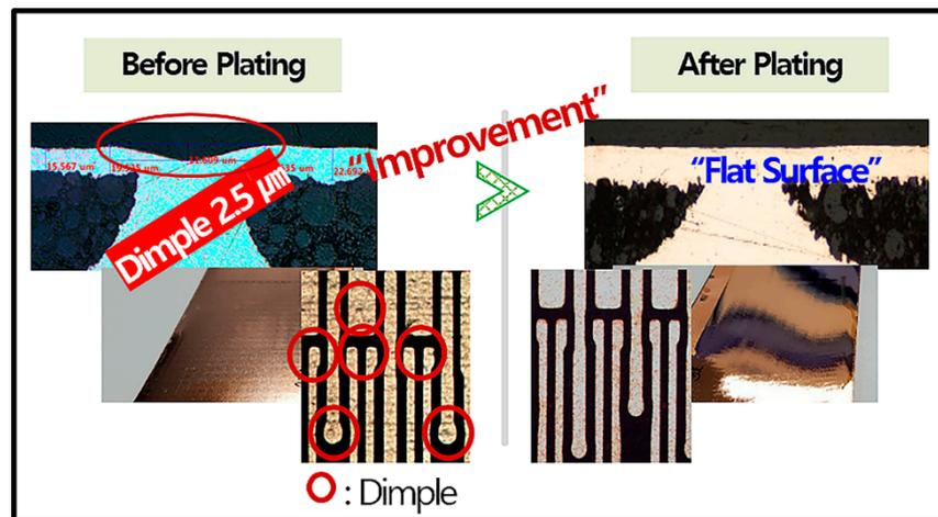
Figure 5. Cu layer flatness before (left) and after (right) Cu plating improvement.
