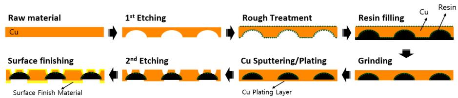
Figure 1. Schematic diagram of two-layer Rt-QFN Manufacturing Process.
