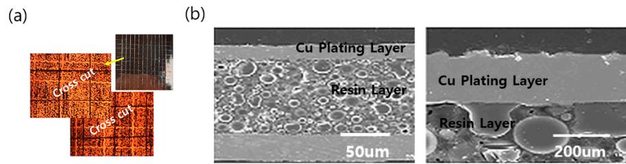
**Figure 8.** Adhesive strength evaluation method: (a) Example photo of Crosscut test; (b) SEM microscope between resin and Cu interface.
