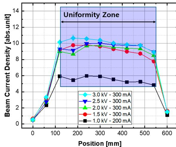
Figure 4. Current density profile of HDS LIS module.
