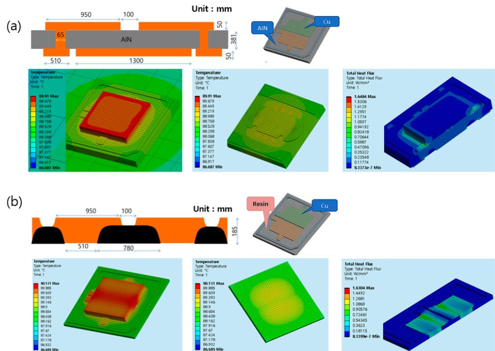
**Figure 12.** Comparison of heat dissipation performance between Ceramic and Rt-QFN substrate: (a) AlN Substrate; (b) Rt-QFN Substrate.
