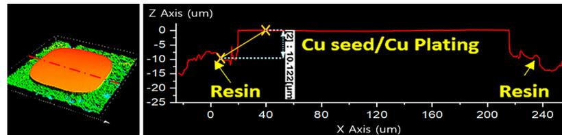
Figure 7. Surface roughness profile of Cu plating layer in two-layer Rt-QFN.
