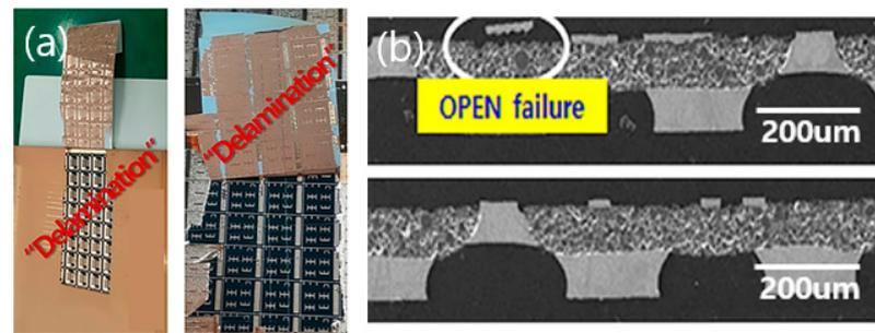
Figure 2. Example of Cu layer peeling failure: (a) Delamination of Cu layer on resin surface; (b) SEM image for the resulting open failure.
