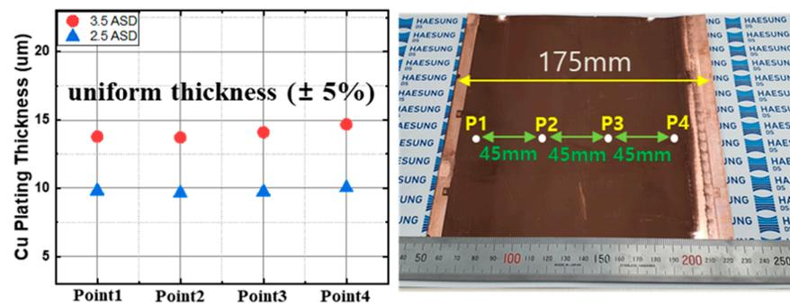
Figure 6. Cu thickness uniformity after Cu plating process.
