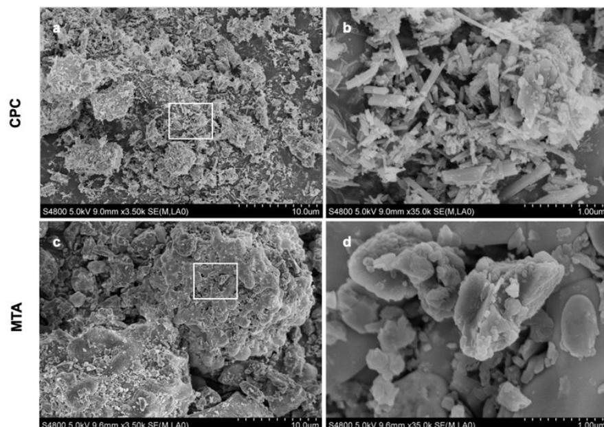
**Figure 1.** Typical SEM images of CPC and MTA powders. The magnifications ranging from  $\times 3.5$  k (a,c) to 35 k (b,d). (b,d) represented the high magnification of the white box in a and c. Scale bar = 10  $\mu\text{m}$  (a,c) and 1  $\mu\text{m}$  (b,d). SEM: scanning electron microscope.
