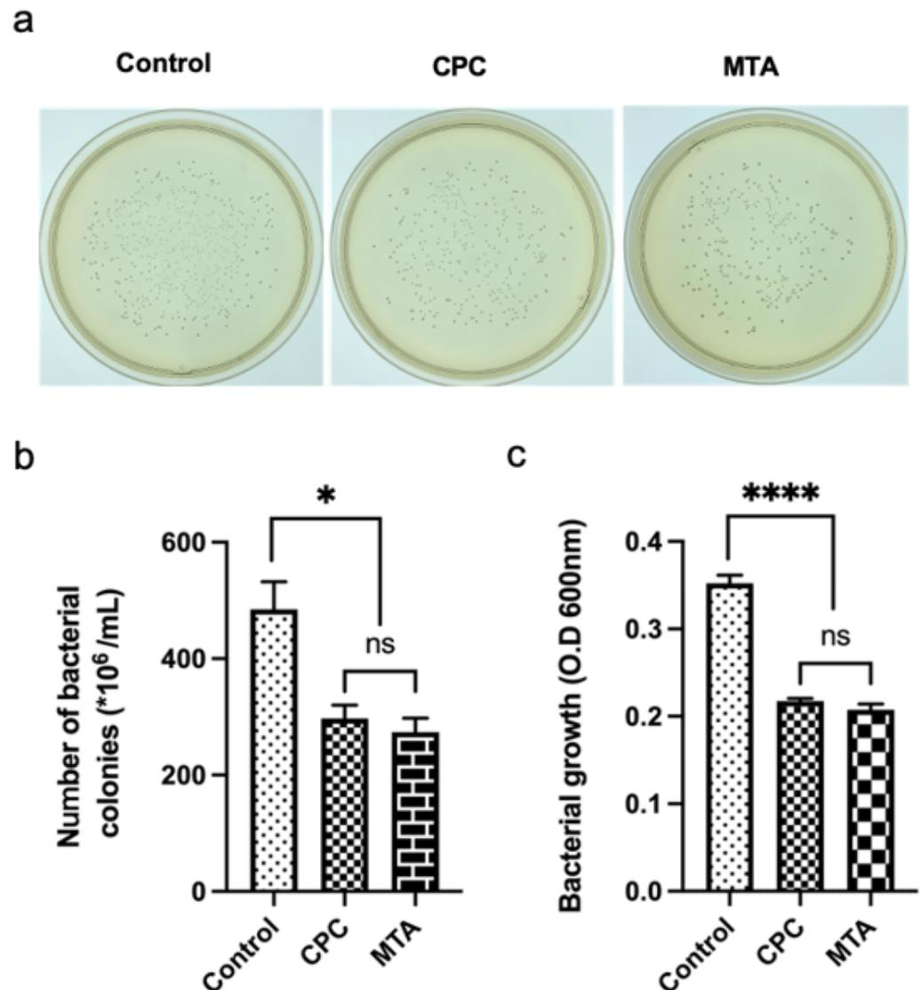
**Figure 2.** Antimicrobial activity of the CPC. Representative plates (a) and the statistical analysis (b) of the CFUs assay. Bacterial growth by DCT assay (c) was measured by a spectrophotometer at 600 nm. Asterisk (\*) indicates a statistically significant difference compared with the control group (\*  $p < 0.05$ , \*\*\*\*  $p < 0.0001$ ).
