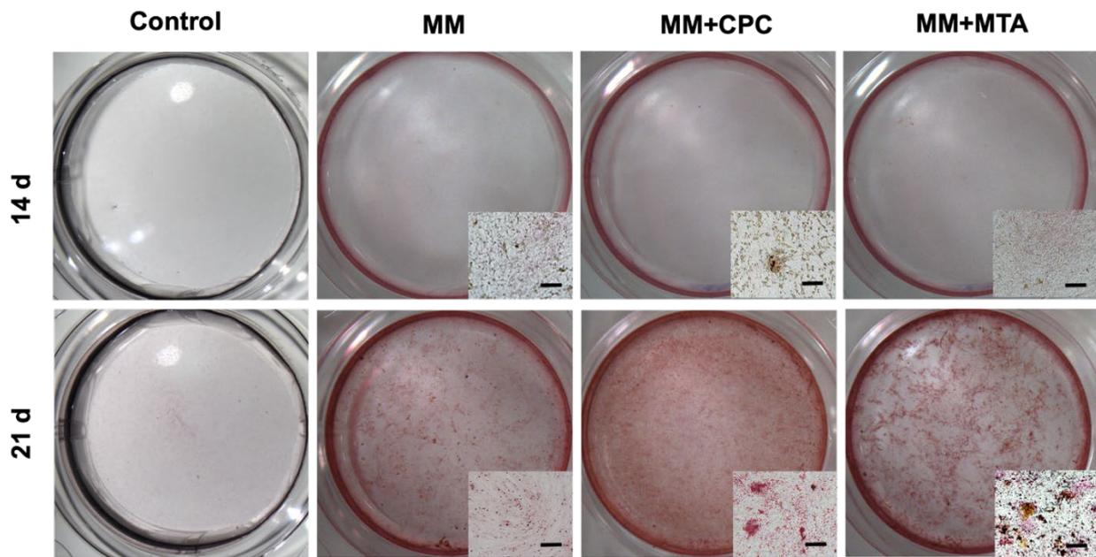
**Figure 4.** ARS of the hDPCs induced by the 0.1 mg/mL CPCe and MTAE with MM for 14 and 21 days. Mineralized nodules formed by induced hDPCs stained red. Pictures were taken by electron microscope and stereomicroscope (bottom right). MM, mineralization medium. Scale bar = 100  $\mu$ m.
