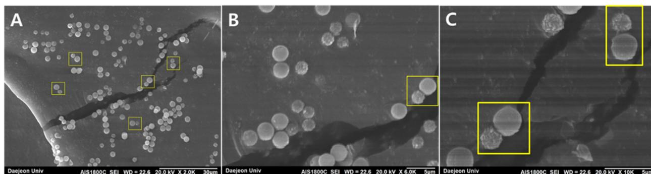
**Figure 4.** SEM images of microparticles of the middle portion of PEG-DEX ATPS after the EDC coupling reaction with different magnifications. (A) 2000 times, (B) 6000 times, (C) 10,000 times magnified. Janus dumbbell particles are shown in yellow boxes. Scale bars are (A) 30, (B) 5, (C) 5  $\mu\text{m}$ . See Experimental for other conditions.
