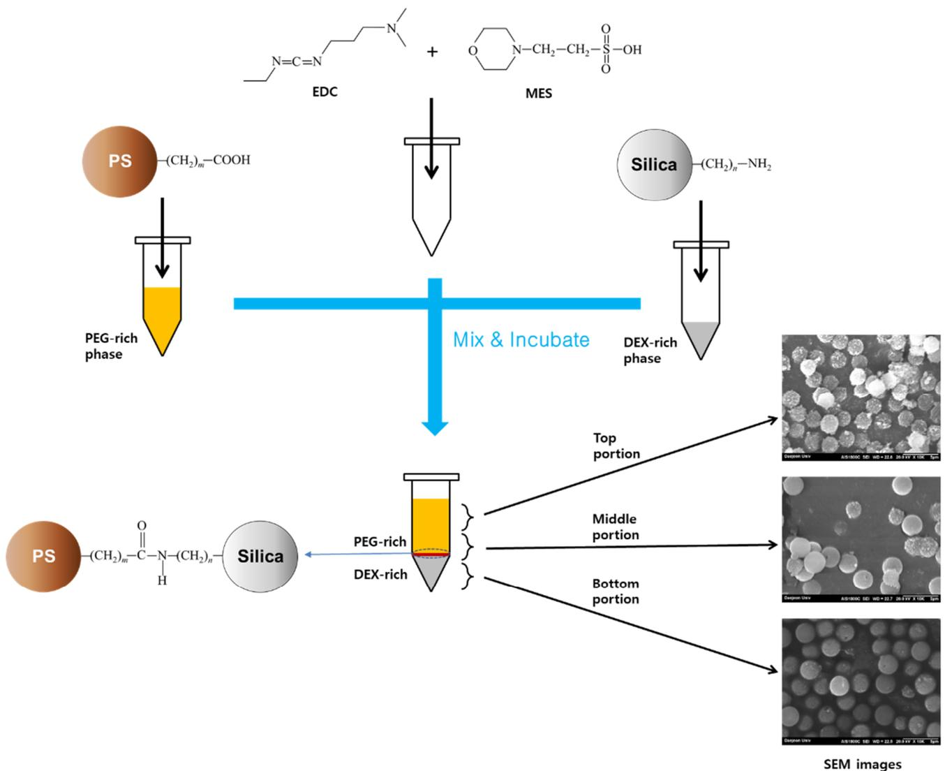
**Figure 2.** Preparation of Janus dumbbell particles in PEG-DEX ATPS. Details were shown in Materials and Methods.
