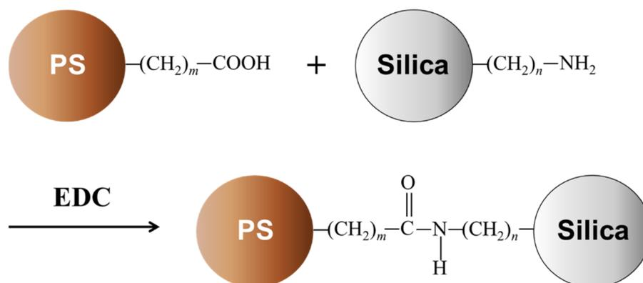
**Figure 1.** Reaction scheme between a carboxyl-activated polystyrene (PS) magnetic particle and an amino-coated silica particle (both from Spherotech®).  $m$  and  $n$  are natural numbers between 2 to 8, according to vendor's information.
