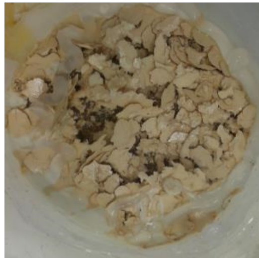
Figure 7. An example of complete degradation of the NBR coating with a filler of rounded particles (NBR-REF) exposed to 30% CH 2 O 2 for 120 days.
