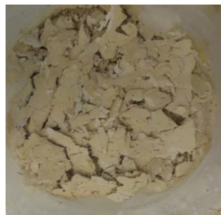
Figure 11. Complete degradation of the NBR-CW coating exposed to 30% CH 2 O 2 for 120 days.
