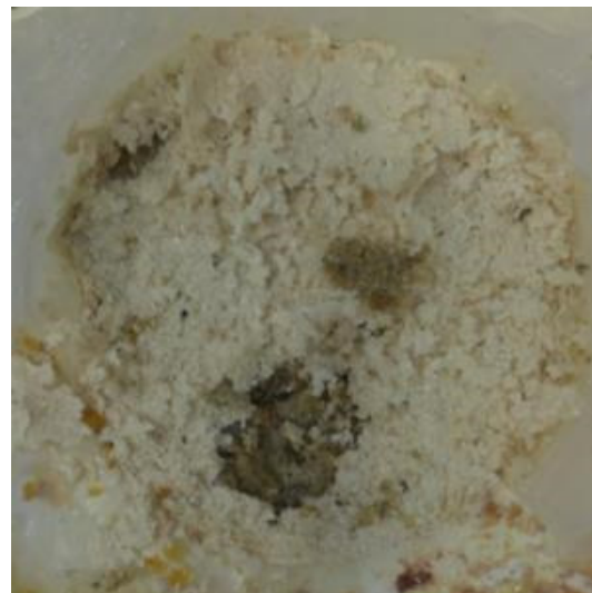
Figure 9. Complete degradation of the NBR-GF coating exposed to 30% \text{CH}_2\text{O}_2 for 120 days.
