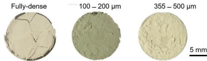
**Figure 2.** Macro-images of the fully-dense and two pores range sizes (100–200 and 355–500  $\mu\text{m}$ ) acquired with an optical microscope.
