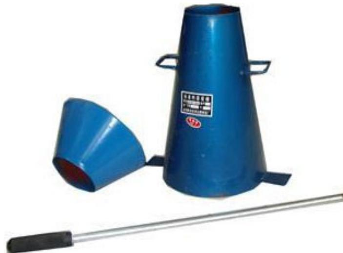
Figure 10. Slump Test Device.
