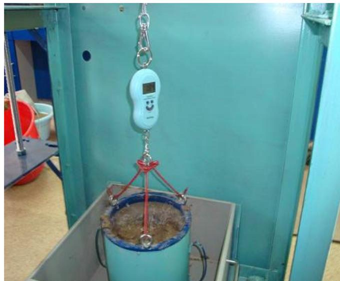
**Figure 9.** Design of Adhesion Resistance Test Device.
