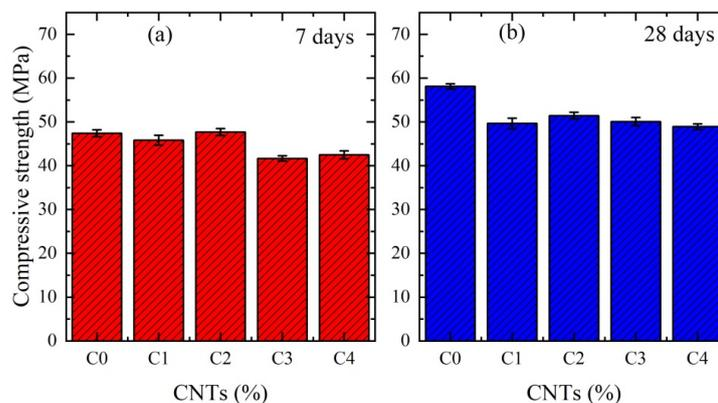
**Figure 3.** Compressive strength of cement mortars with different wt.% of MWCNTs. The results are for 15 min of sonication time without surfactant. (a) for 7 days, (b) for 28 days.
